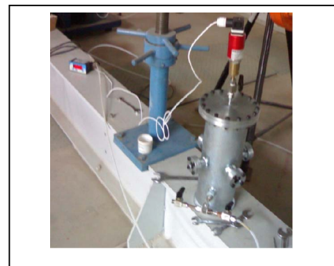
Figure 3. Calibration gas chamber with pressure gauge.
