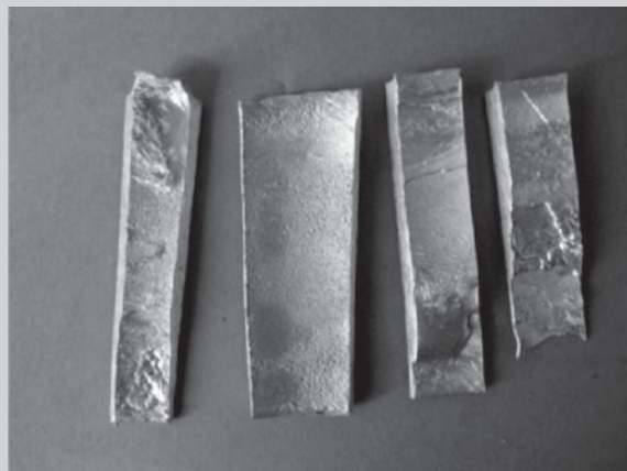
Figure 4. Al-12Si casting (4 mm thick): (a) 600 rpm, (b) 800 rpm, (c) 1,000 rpm, (d) 1,200 rpm (L-R, respectively).
