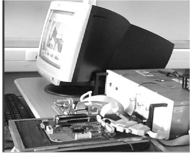
Fig. 12. FPGA Based PID Controller Setup.
