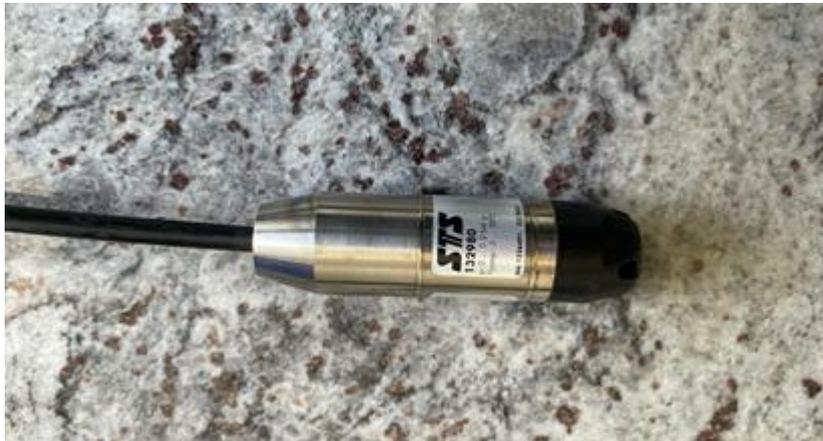
Figure. 3.4: A closer view of the Pressure Transducer.
