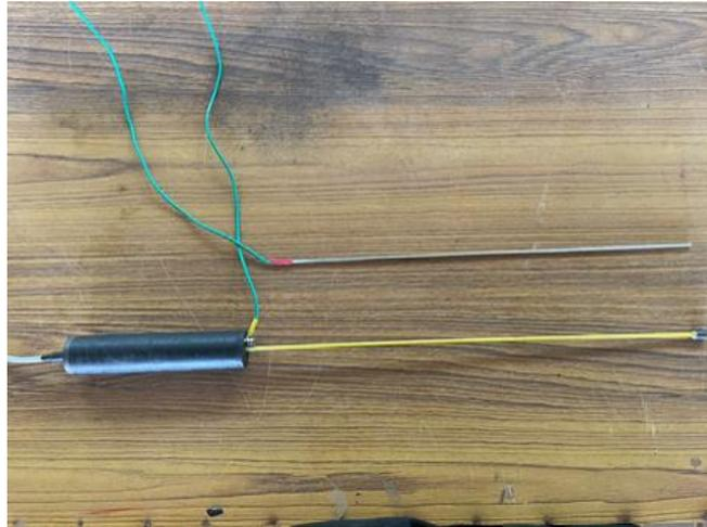
Figure 3.2: Capacitance-type wave meter
