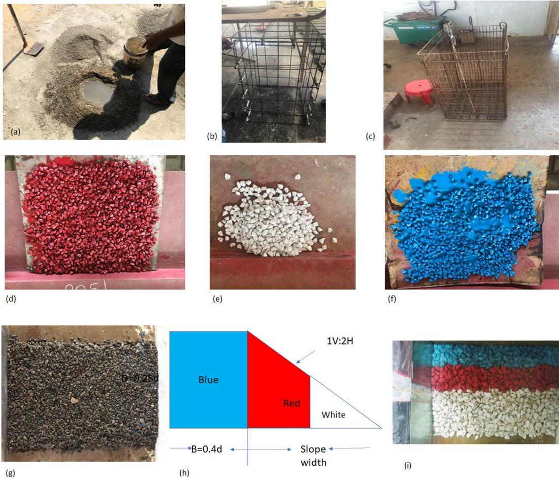
Plate 3.4: (a) - Aggregate mix, (b) & (c) – Preparation of mesh of vertical wall, (d), (e), (f) - Armour units for the protection of toe, (g) – Bedding Layer or base layer on flume bed, (h)- arrangement of a toe, (i)- Vertical wall with the protection of toe.
