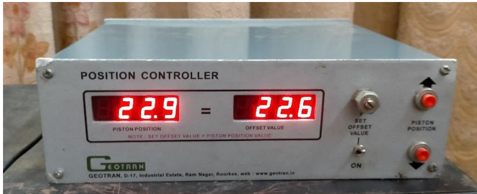
Figure 3.11 View of the Position Controller
