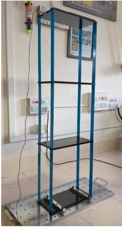
Figure 1.7 (a) Frame structure, (b) Liquid damper on a frame structure
