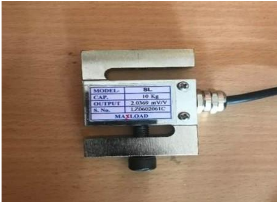
Figure 3.5 View of the S-type Load cell
