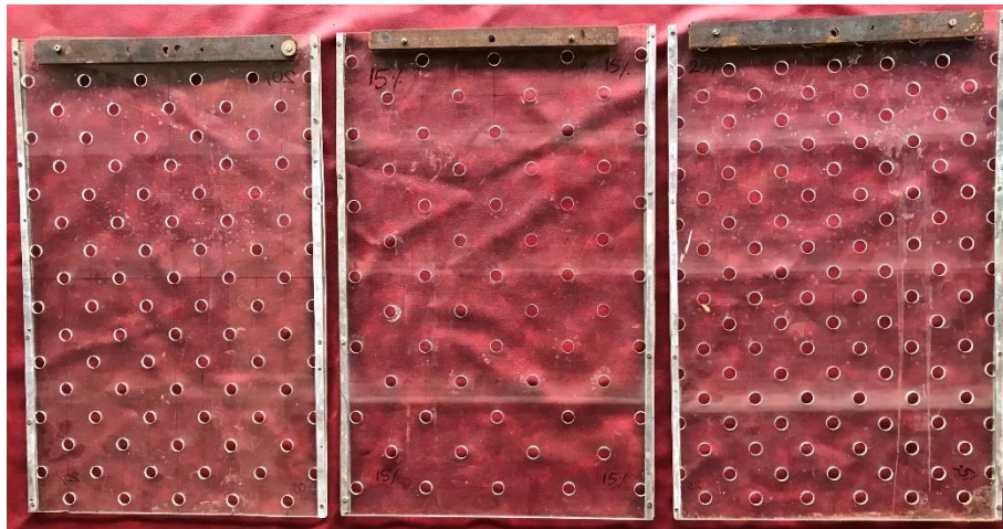
Figure 3.13 view of porous baffles with hole arrangements
