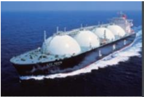
Figure 1.3 Moss-type LNG carrier (source: MODEC, Inc.)
