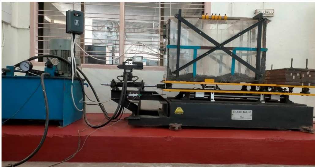
Figure 3.10 view of experimental shake table setup
