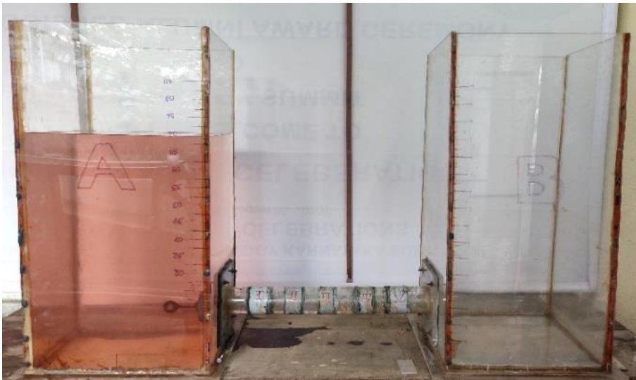
Figure 3.18 Experimental setup, water is stored in one tank with a known head
