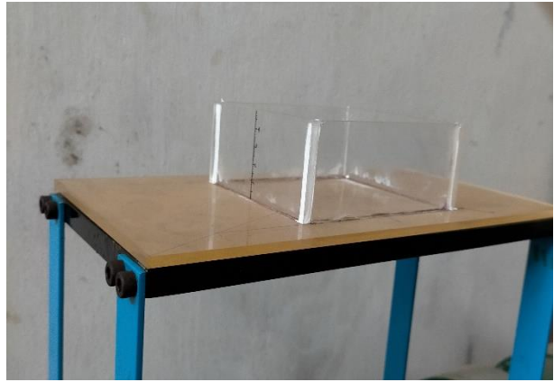
Figure 1.7 (a) Frame structure, (b) Liquid damper on a frame structure
