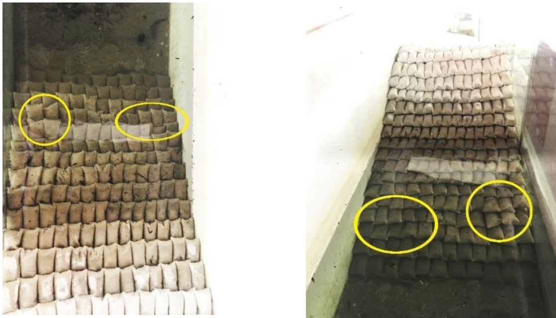
Fig. 4.14 Bag 1 configuration subjected to 0.12 m high waves with 2.2 s time period for a relative water depth of 0.008 < d/gT^2 < 0.020 (i.e. 0.40 m water depth). Highlighted armour units exhibited sliding instability due to uplifting.
