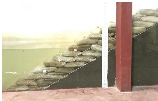
Fig. 4.28 Constructed model of double-layer GSC breakwater structure.
