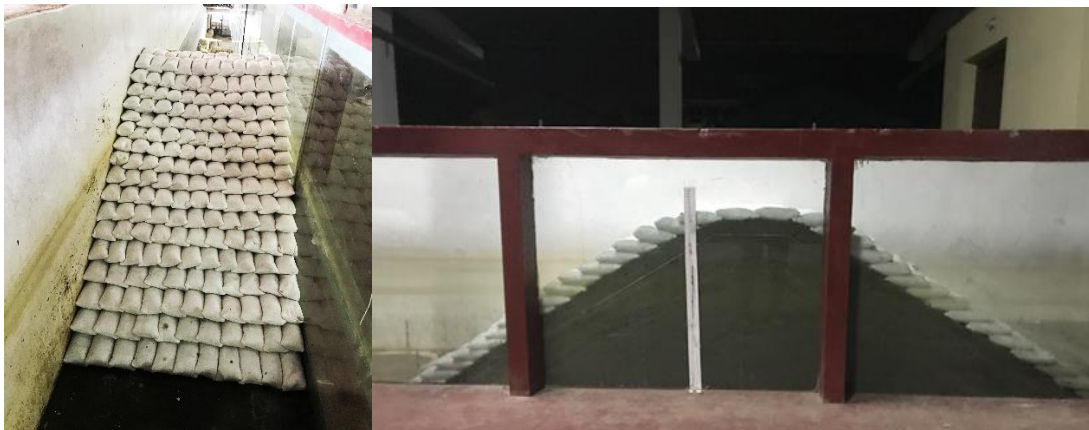
Fig. 4.1 Single-layer GSC breakwater model after construction at wave mechanics laboratory
