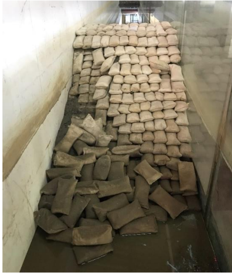
Fig. 4.37 Total Failure (DC4) after exposure to 0.16 m wave heights.
