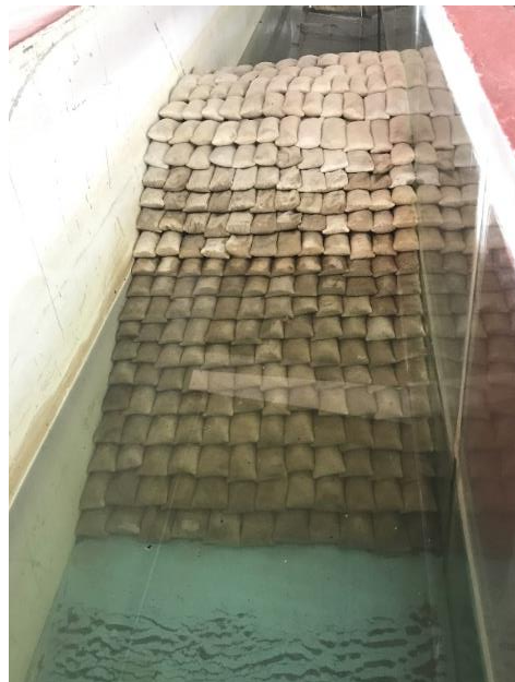
Fig. 4.36 Bag 1 Double-layer configuration, Stable (DC0) after exposure of 0.06 m wave heights
