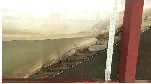
Fig. 4.29 Constructed model of double-layer GSC breakwater structure with slope-parallel outer layer.
