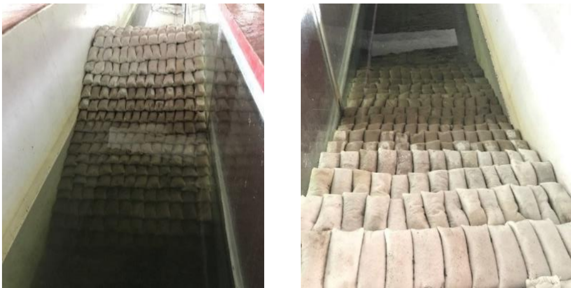
Fig. 4.13 Stable structure ('Bag 1') subjected to attack of 3000 waves of time period 2.2 s, (a) wave height 0.06 m and (b) wave height 0.08 m, for relative water depth 0.008 < d/gT^2 < 0.020 (i.e. 0.40 m water depth).
