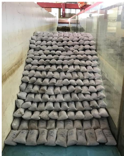
Fig. 4.52, Image showing sand container filled to 15% cement and arranged to a single layer. Note the bulkiness of the units contributing higher porosity.
