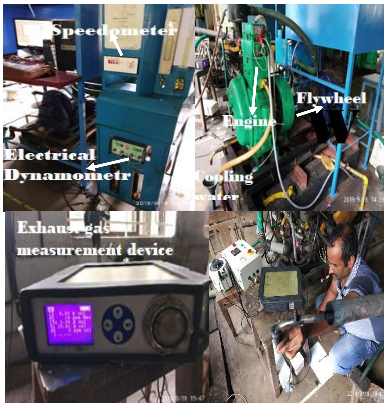
Figure 3.8 Pictorial view of the engine test set-up
