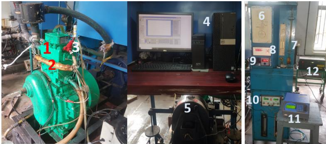
1) Kirloskar TV 1 engine, 2) Fuel line with heater, 3) Fuel injector 4) Computer system, 5) Eddy current operated dynamometer, 6) Control panel, 7) Fuel consumption indicator, 8) Engine speed indicator display, 9) Temperature indicator, 10) Engine load controlling unit, 11) Gas analyzer, 12) AVL smoke analyzer
