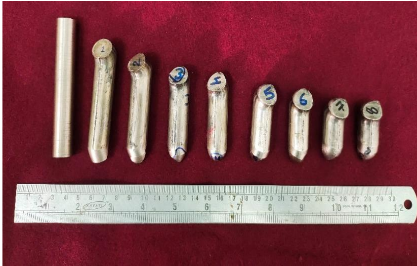
Figure 8.6 ECAP processed C70600 alloy
