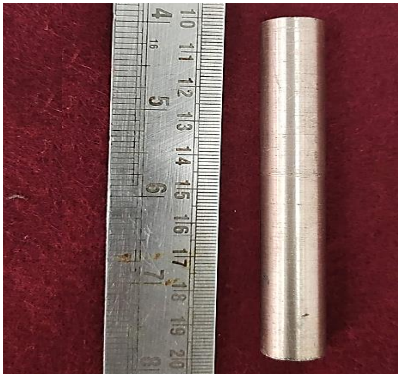
Figure 8.2 Machined sample of C70600 to execute ECAP
