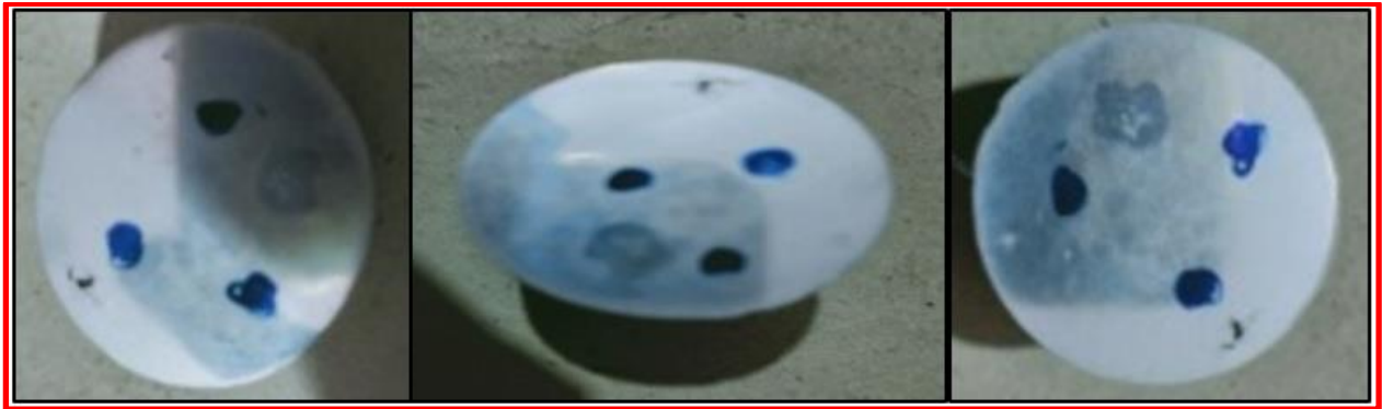
Figure 5.11: Images of micro hardness test specimens of spray deposited Al-Si alloy matrix composite reinforced with a) 5% b) 10% c) 15% ZrO 2 particles for 12.5 wt. % of Silicon
