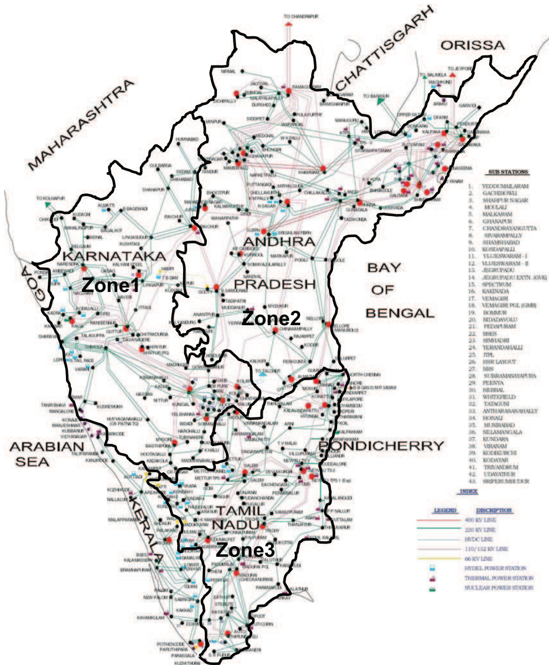
Figure 6.9: Geographical map of 72-bus equivalent system of Indian southern region power grid
