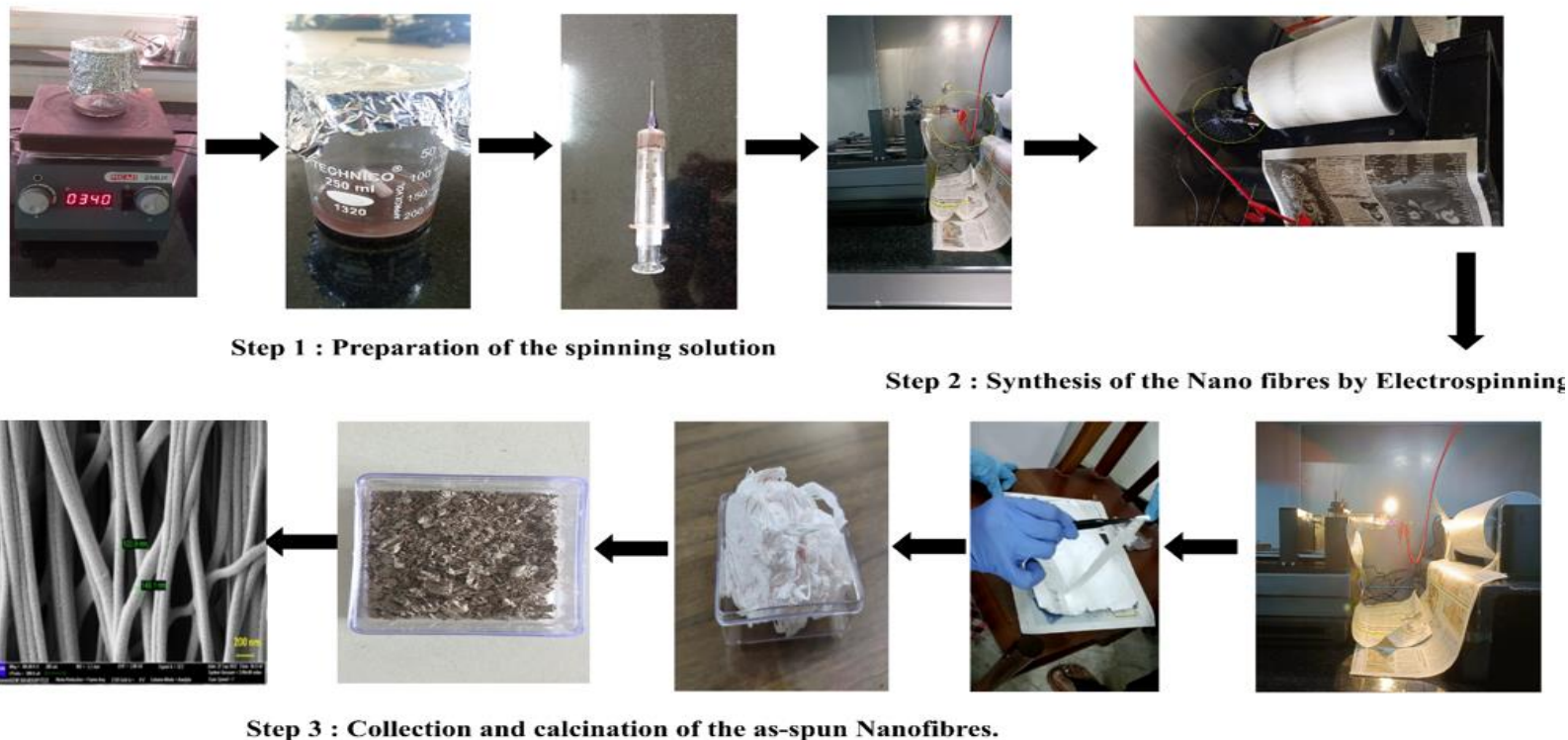
Figure 3.3: Electrospinning technique to develop transition metal doped Ce-Pr catalysts
