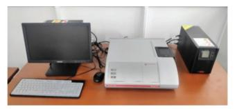
Particle Sizing and Zeta Potential Analyzer
