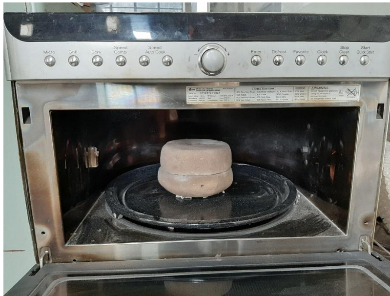
Figure 3. 2 Experimental set up of microwave hybrid heating mechanism.
