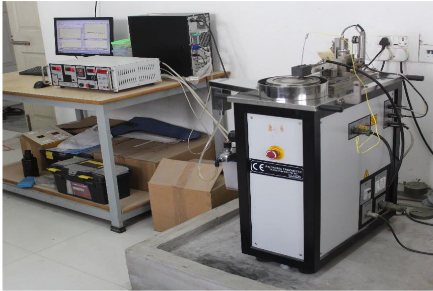
Figure 3. 4 Pin on disc tribometer experimental set up.
