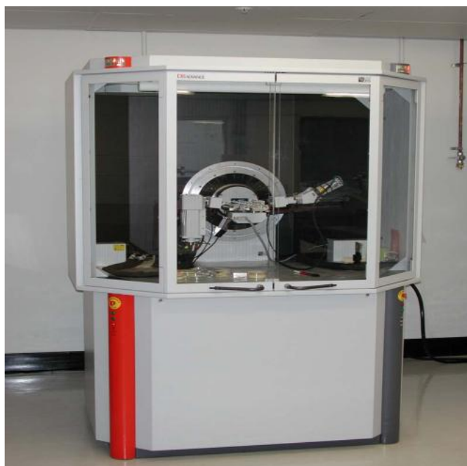
Fig 3.13 X-ray diffraction operated at 20 mA and 30 kV with Cu- k\alpha radiation
