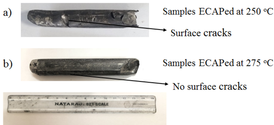
Fig 3.4 ZE41 Mg samples ECAPed at a) 250 °C and b) 275 °C.
