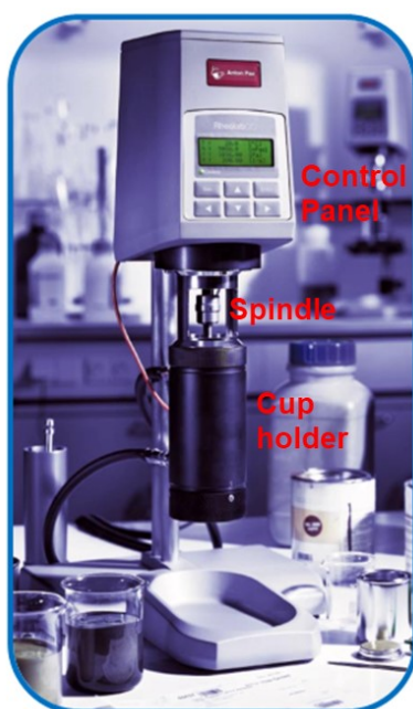
Figure 3.8. Rotational Rheometer (Anton Paar™: Rheolab C-LTD180/QC), NIT Warangal.
