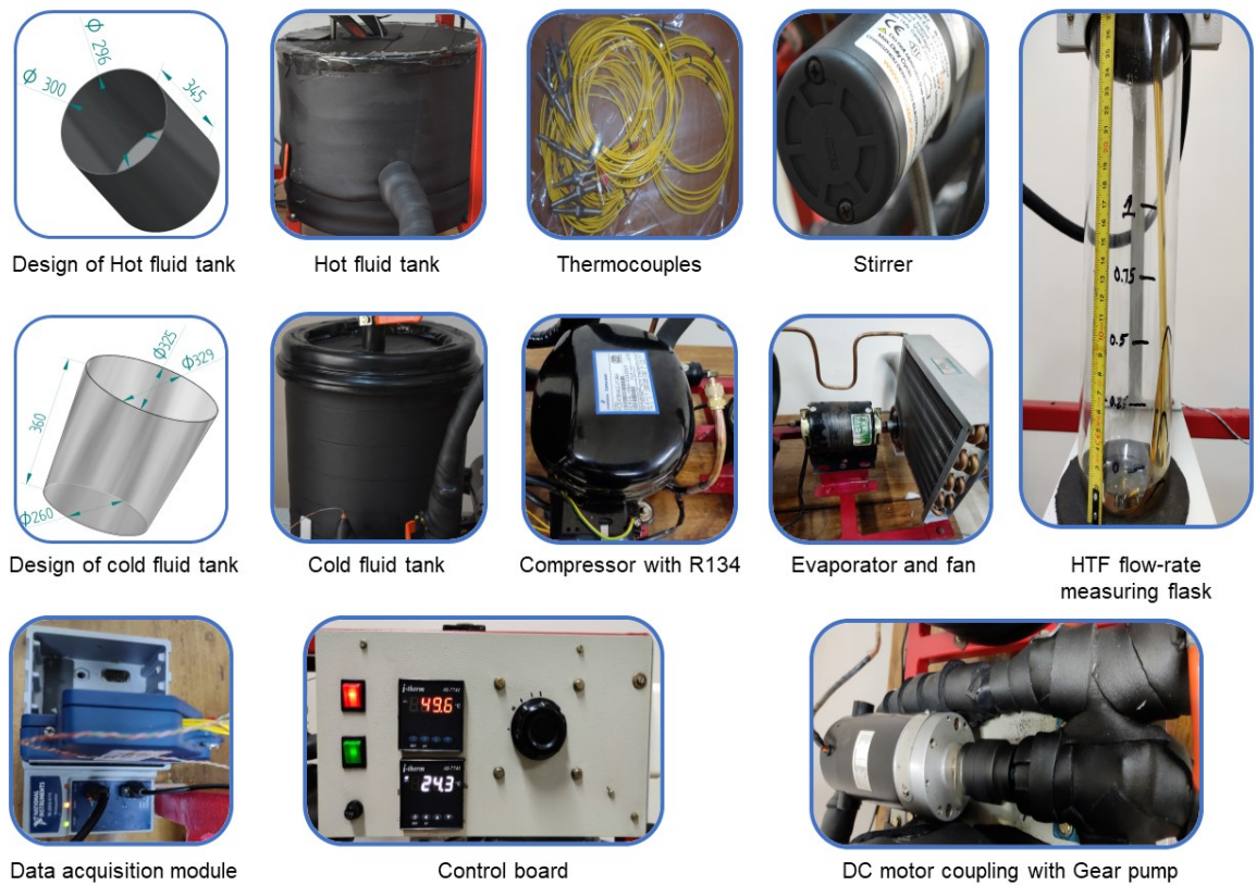
Figure B.2. Design of HTF tanks and individual parts of shell-tube LHTES unit.
