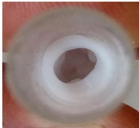
Figure 4.4. PCM cavity formation inside the tube during the cooling process.
