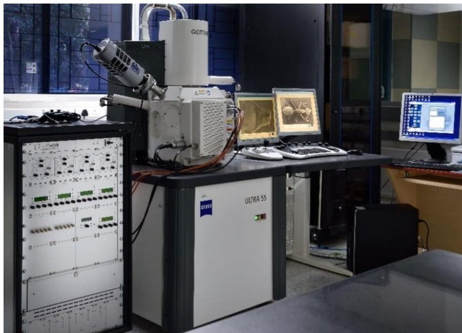
Figure 2.6 Carl Zeiss Ultra 55 FESEM used for our study (Image courtesy: CeNSE, IISc Bangalore).
