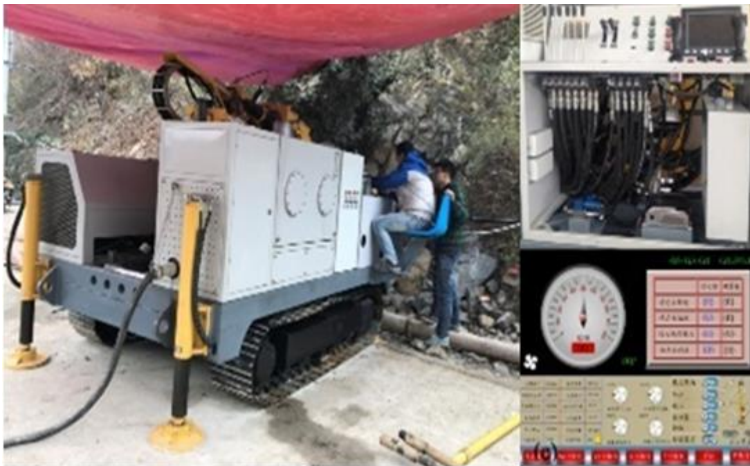
Fig.1.1 An overview of the drilling process monitoring apparatus (DPM)
