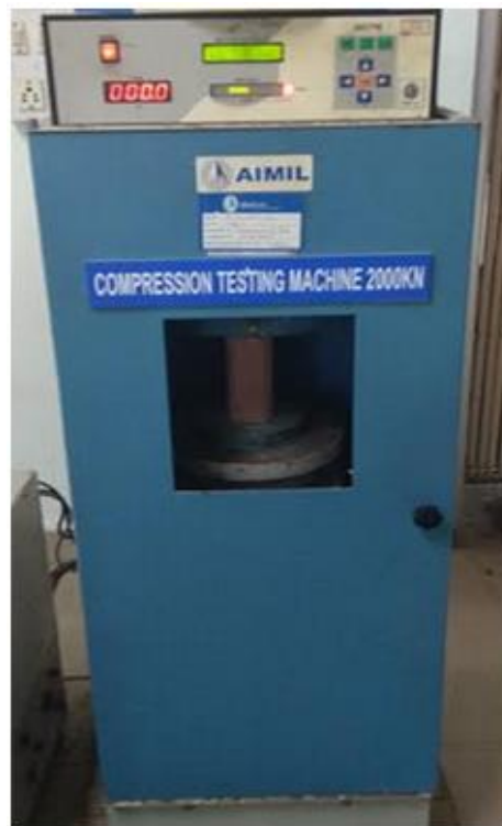
Fig. 3.14 UCS testing machine
