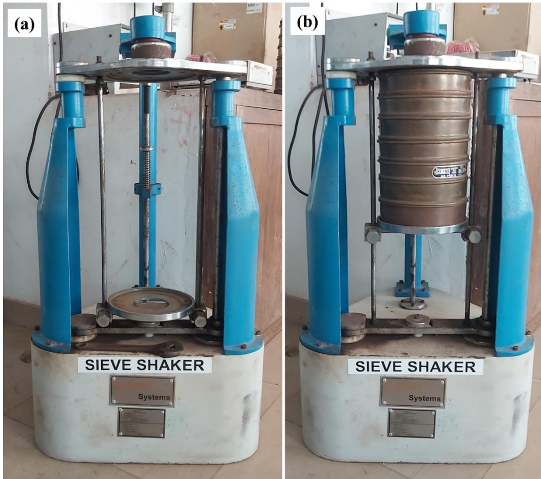
Fig. 3.2: (a) Ro-Tap sieve shaker, and (b) Ro-Tap sieve shaker with standard test sieves.
