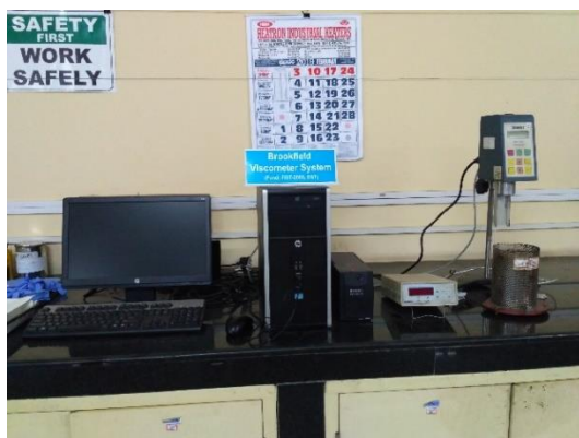
Figure 3.2 Rotational viscometer apparatus
