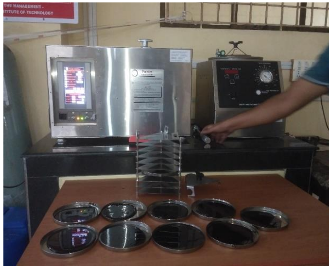
Figure 3.9 PAV apparatus and samples
