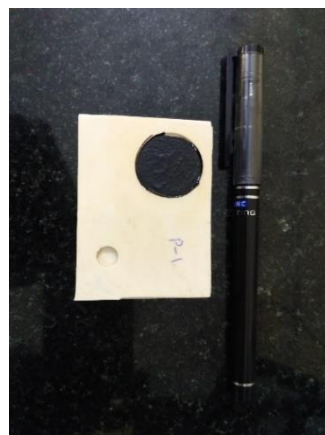
Figure 3.7 Silicon mould holding 25mm dia. sample
