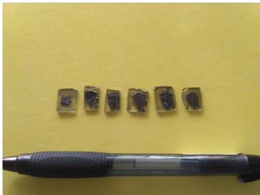
Figure 3.12 SEM Specimens prepared without slanting slide
