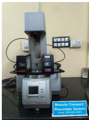
Figure 3.6 DSR Apparatus (MCR-502)
