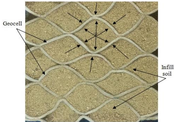
Fig. 5.26 Confining effect of geocell reinforced sand
