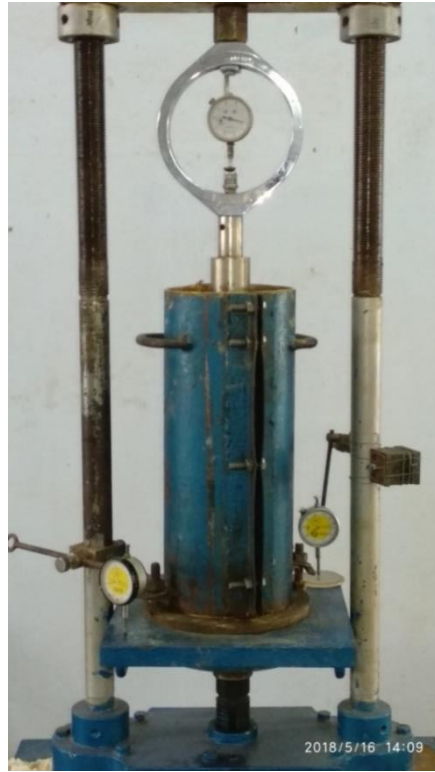
Fig. 4.8 Load tests on stone columns in a unit cell
