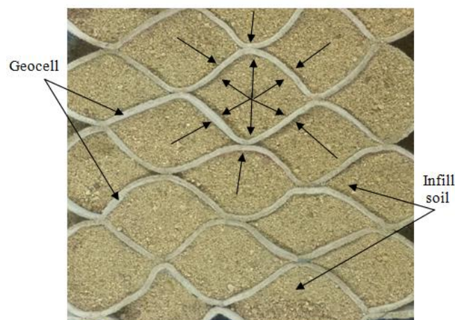
Fig. 1.2 Confinement of soil using geocell
