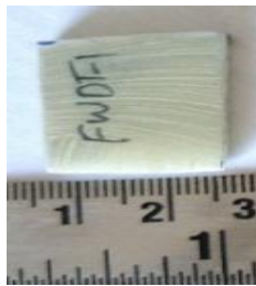
Figure. 3.8 Density test sample
