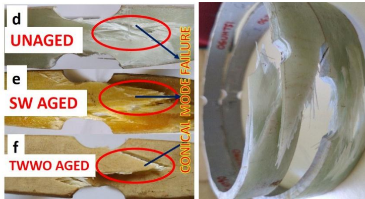
Figure:B1.4 Samples tested for hoop tensile strength (d-unaged tested sample, e-sea water aged tested sample, f-tap water with oil aged tested sample)
