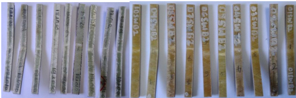
Figure:B1.6 Bending tested samples
