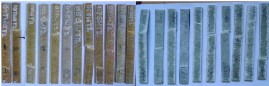
Figure:B1.5 Tensile tested samples
