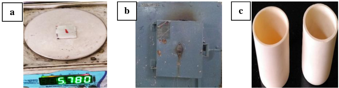
Figure 3.9 Ignition test set up: (a) Ignition test sample weighed before the test, (b) Muffle furnace(burning of samples inside furnace), (c) Alumina crucible(sample kept in a furnace with this crucible)
