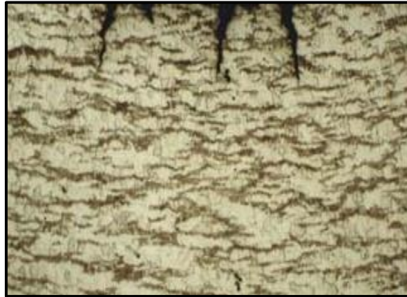
Fig. 1.4 Corrosion Fatigue Cracks (www.hghouston.com)
