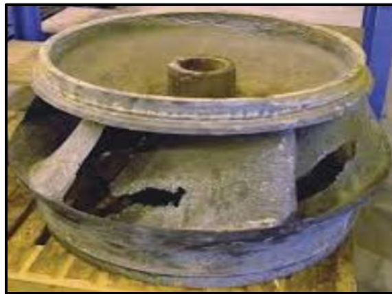
Fig. 1.1 Corrosion of Pump Impeller in Sea Water ( www.tomson.com )
