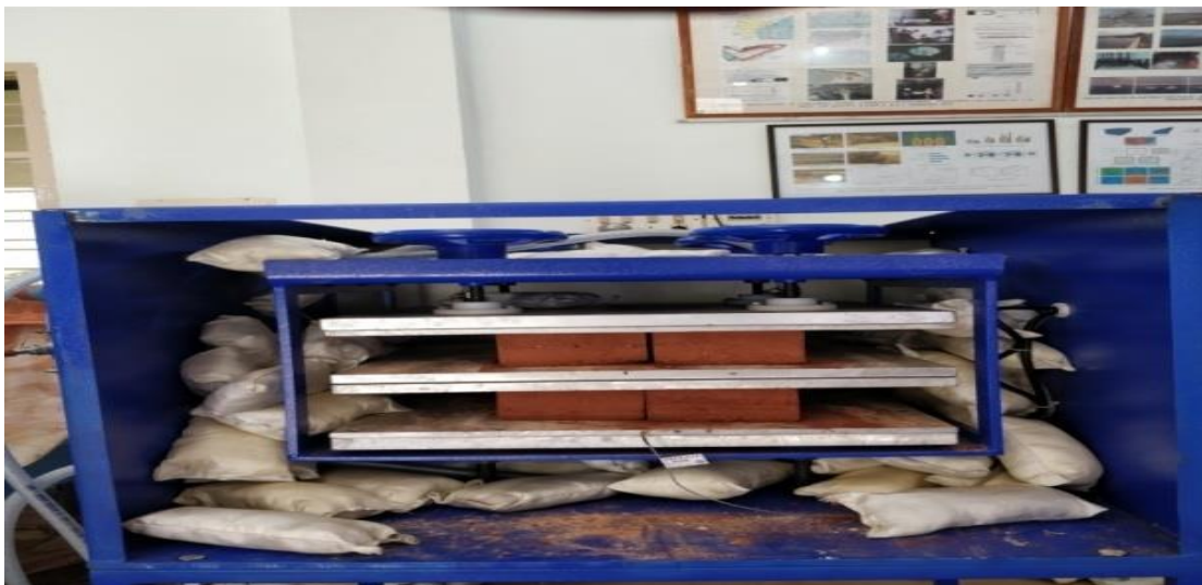
Figure 3.7 A view of thermal conductivity apparatus
