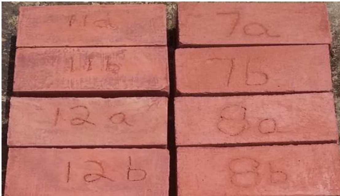
Figure 1.6 Bricks with IOT, sand and cement
