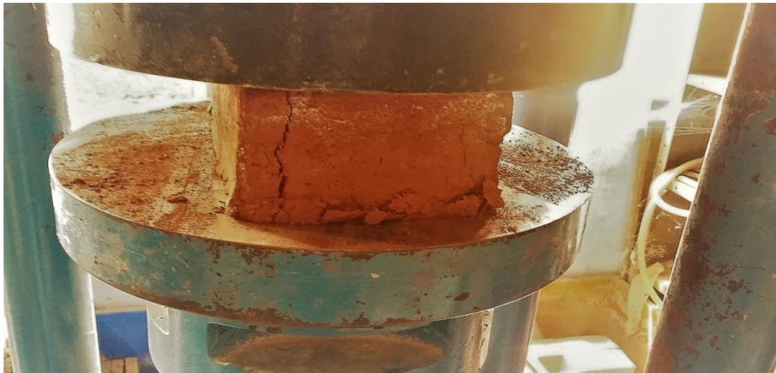
Figure 3.5 Illustration of compression test on IOT – Perlite brick
