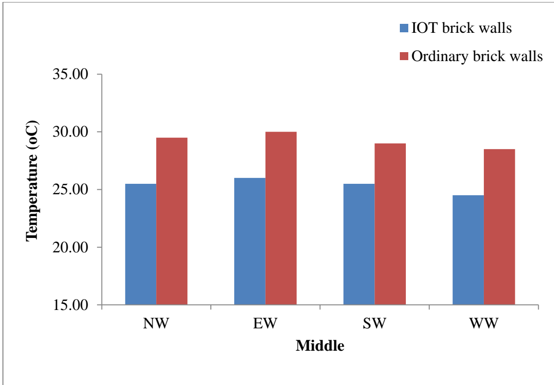
Figure 4.14 Temperature measured from 8am to 10am at middle of the outside walls
