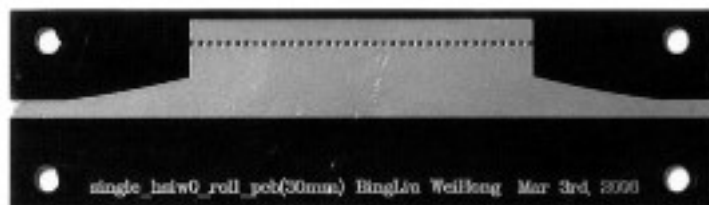
Figure 2.13: Fabricated prototype of HMSIW.
