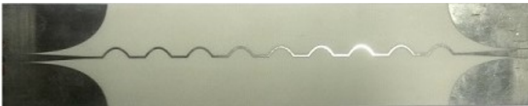
Figure 3.6: Fabricated prototype of the proposed Goubau line.
