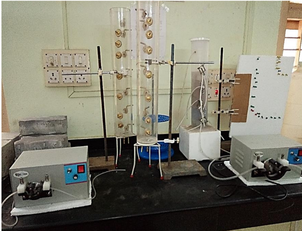
Figure 3.3 Laboratory Scale Acrylic Column Filters
