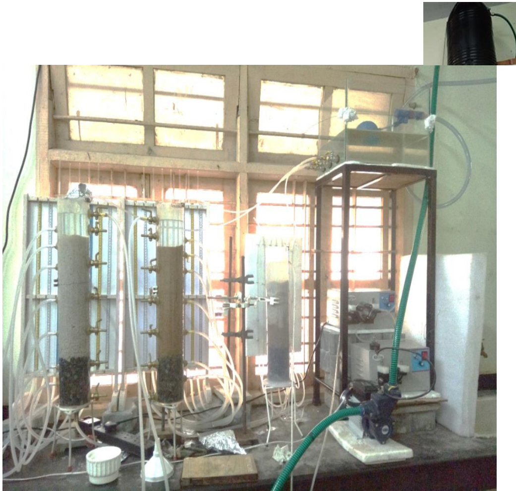
Figure 3.7 Experimental Set-up with Constant Head Tank
