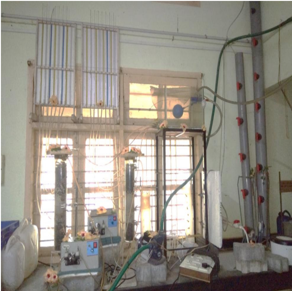
Figure 3.9 Experimental Set-up with Backwash Arrangement
