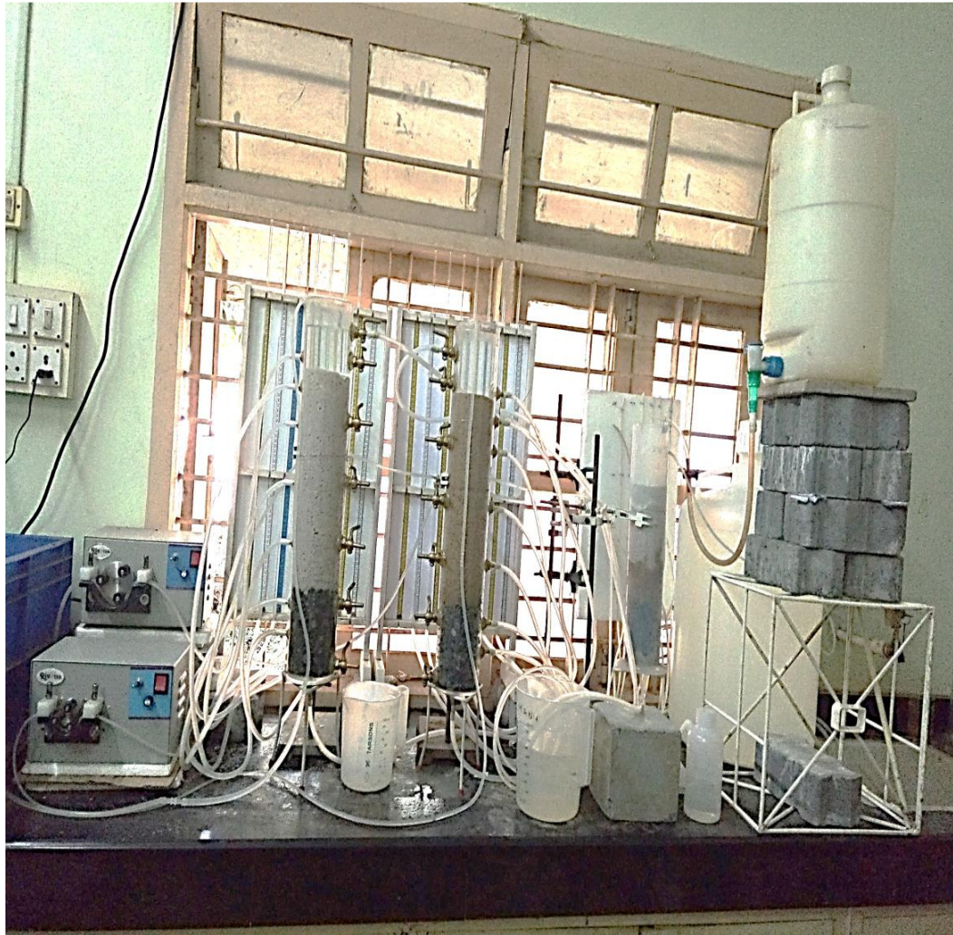
Figure 3.6 Experimental Set-up of Slag and Sand Filters for Small Flowrate
