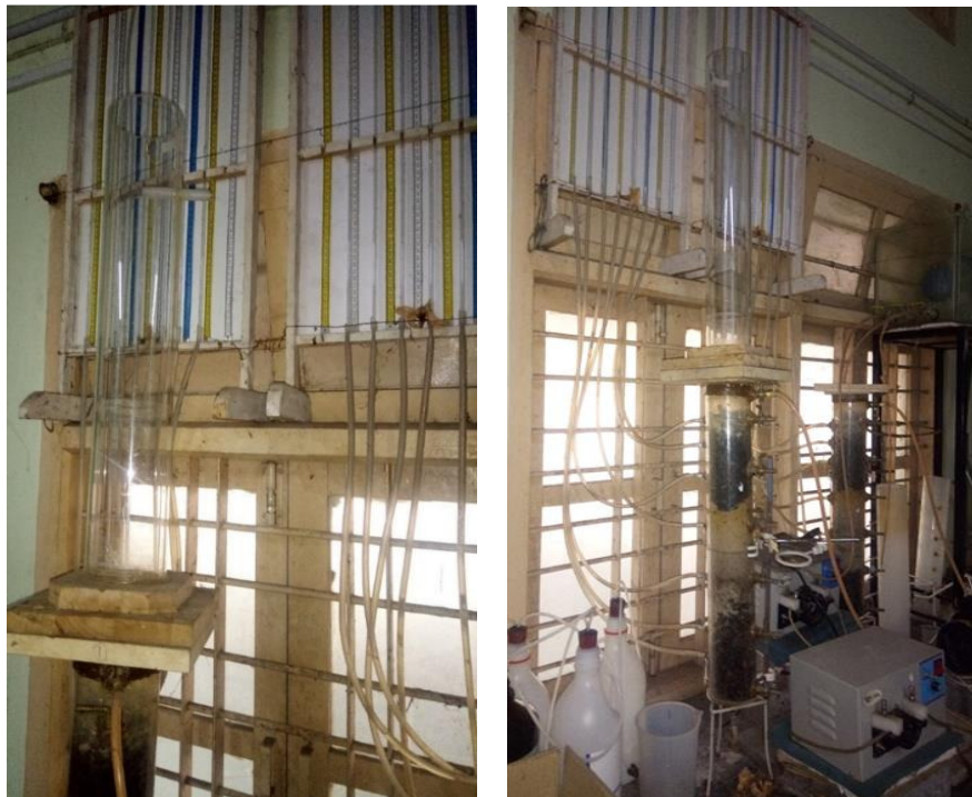
Figure 3.8 Filter Backwash Arrangement
