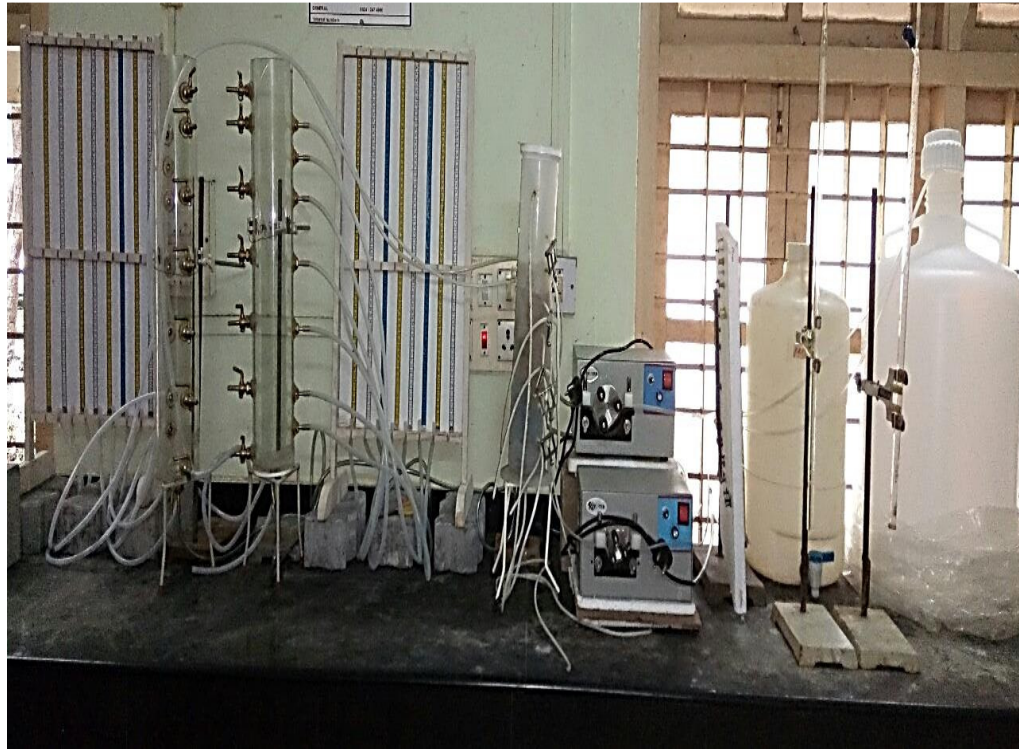
Figure 3.4 Experimental Set-up of Filters with Manometer
