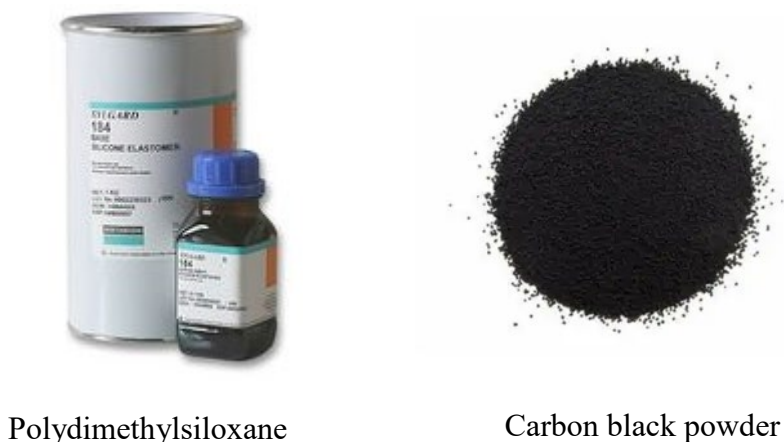
Figure 2.3 Procured polymer and filler materials
