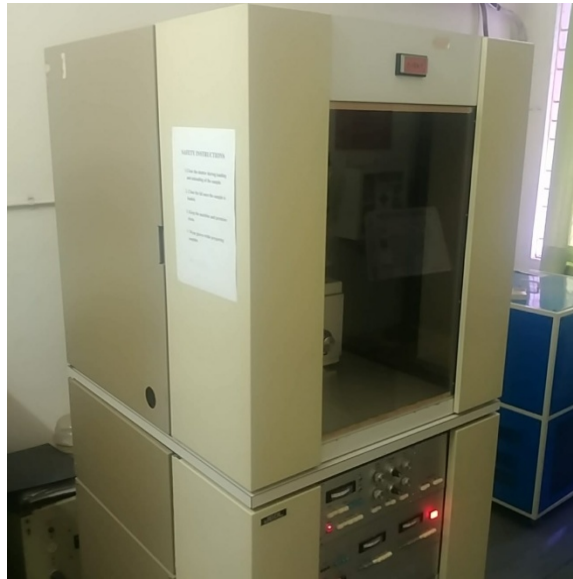
Figure 2.22 X-ray diffractometer measuring instrument (JDx8P, JOEL model)
