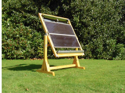
Figure 1.14 Prototype of solar tracker using two bimetallic strips. (Clifford and Eastwood 2004)
