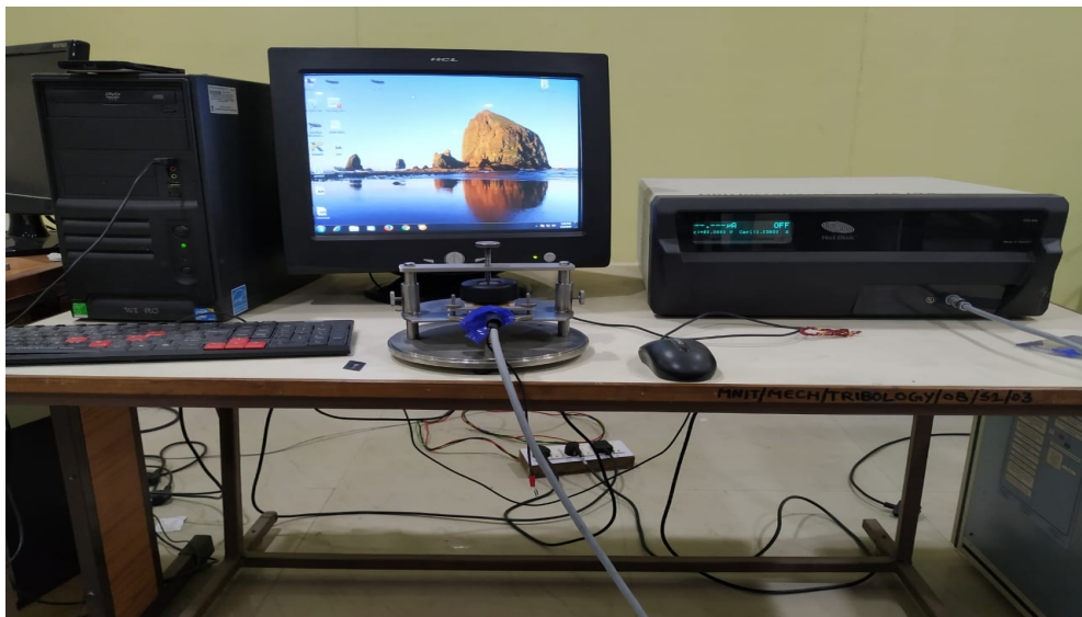
Figure 2.20 Hot Disk TPS thermal constants analyzer setup
