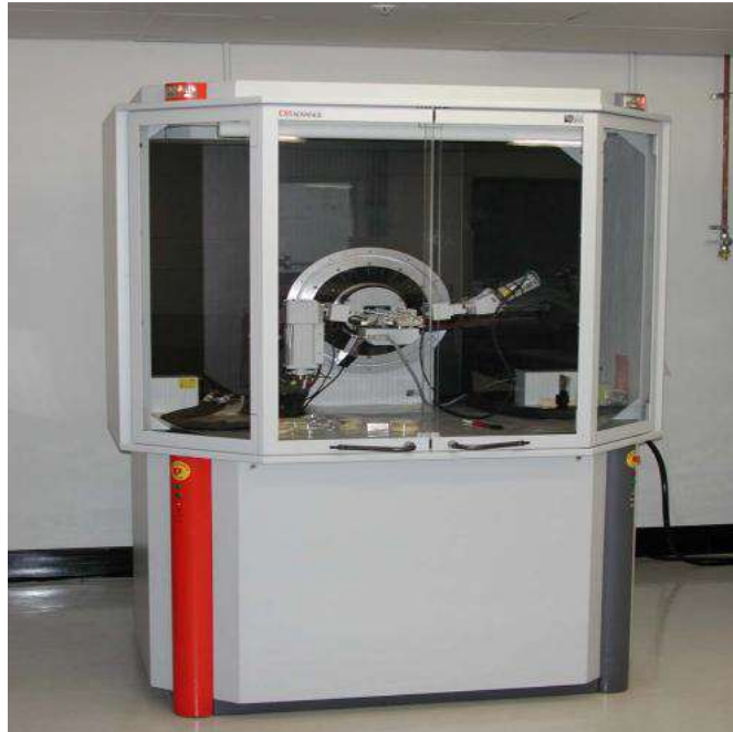
Figure 3.10 X-ray diffraction operated at 20 mA and 30 kV with Cu- \alpha radiation
