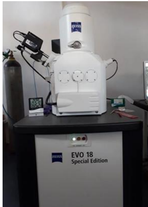
Figure 2.8 Set up for SEM characterisation of the composites
