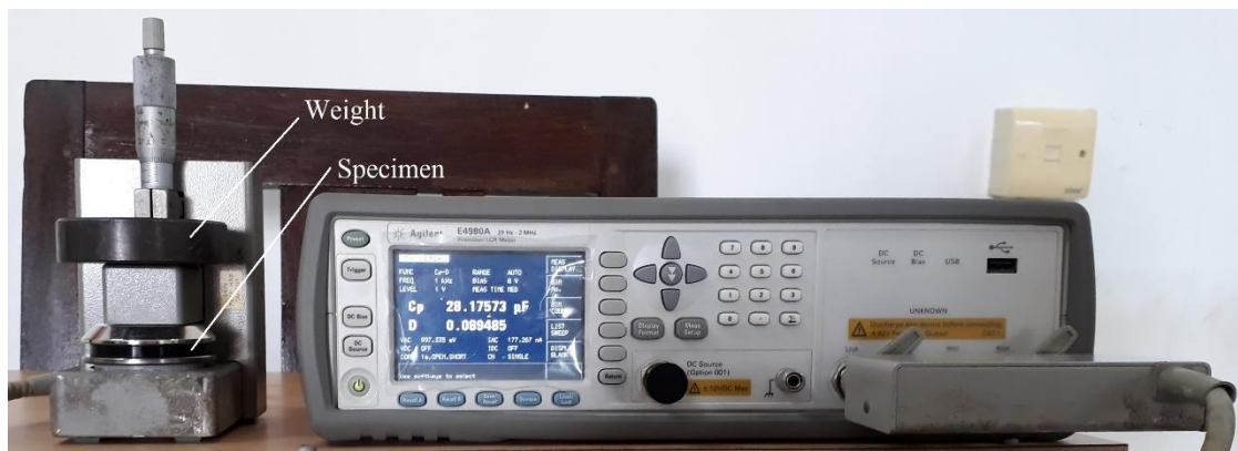
Figure 2.12 Setup for determining the piezoresistive and piezo capacitive characteristics
