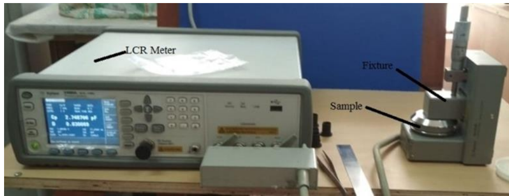
Figure 2.11 Test set up for determining dielectric properties of the composite specimens
