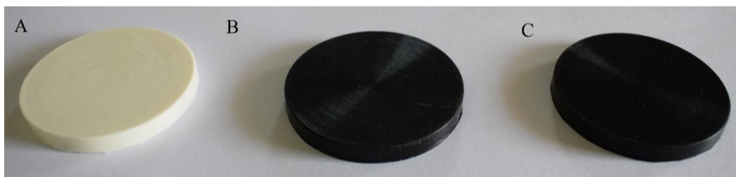
Figure 2.7 Composite samples for dielectric and electromechanical tests (A: DDC, B: CDC and C: CDDC)
