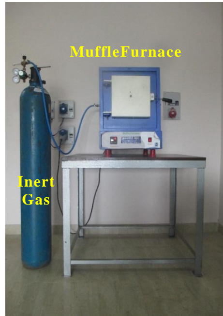
Figure 3.9 Muffle Furnace with inert gas setup.
