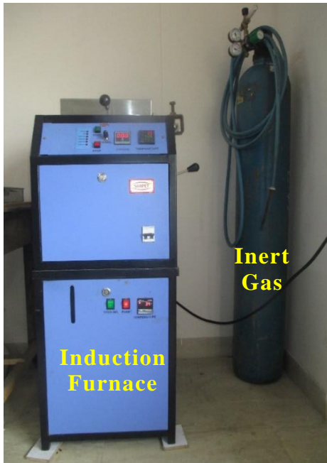
Figure 3.8 Induction melting furnace with inert gas setup.
