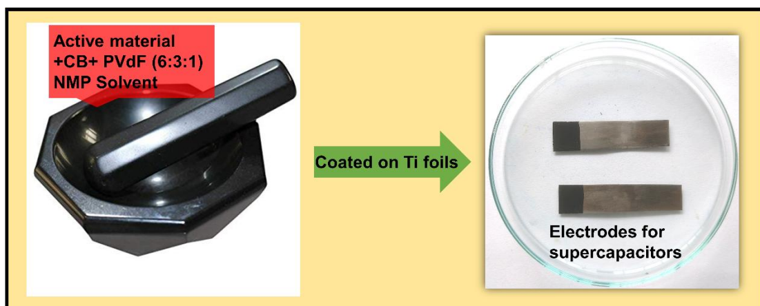
Figure 2.7 Schematic of electrodes preparation for supercapacitors.
