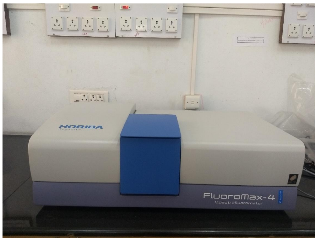
Figure. 2.12. Horiba scientific Fluoromax-4-spectrophotometer instrument used for the PL studies.
