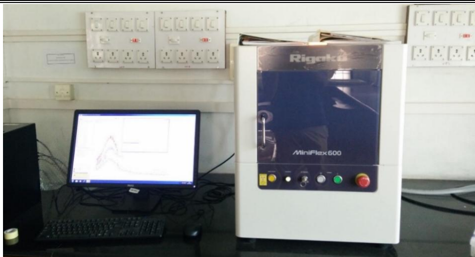
Figure. 2.5. Powder X-ray diffractometer (Rigaku MiniFlex600).
