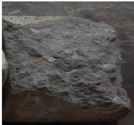
**Fig 6.3 OPCC specimen spalled during the exposure to 600°C**
