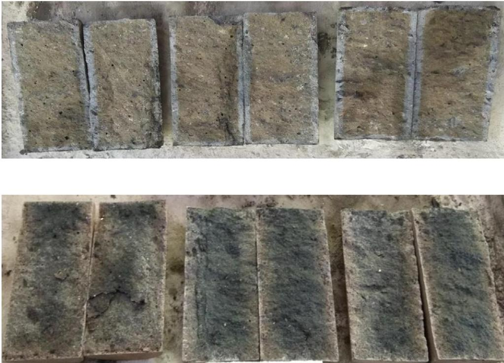
**Fig 5.22 Typical HSAASC mix specimens after the bulk diffusion test.**
