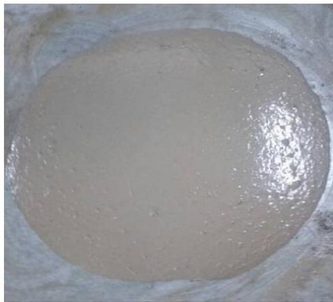
**a – Slump Flow Test**
