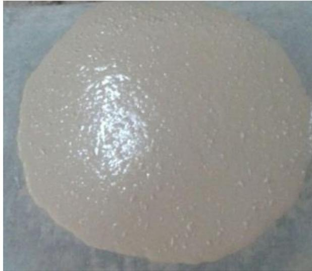
Fig 4.3 Slump flow of AASC mix with sodium phosphate placing after 20 minutes
