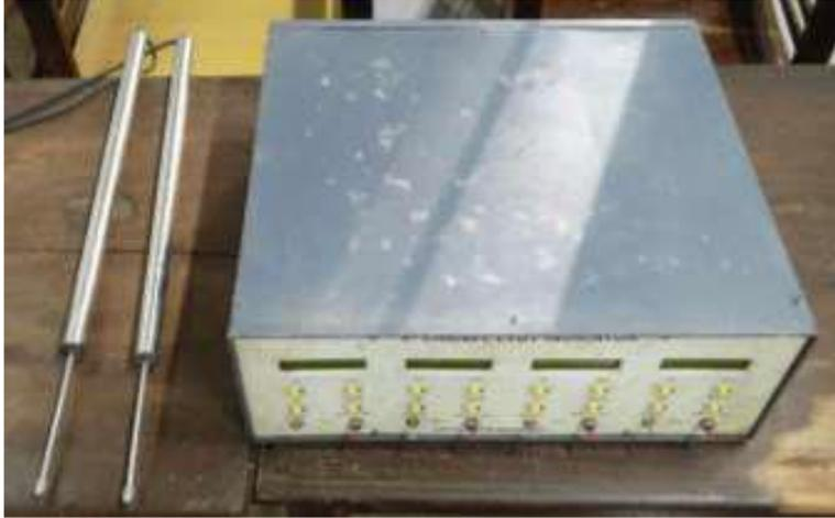
**Fig 8.4 LVDTs along with the data acquisition system**
