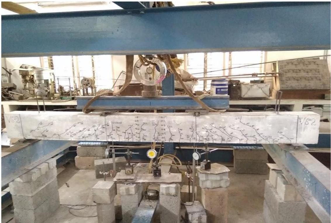
**Fig 8.3 Experimental setup for the testing the beams**
