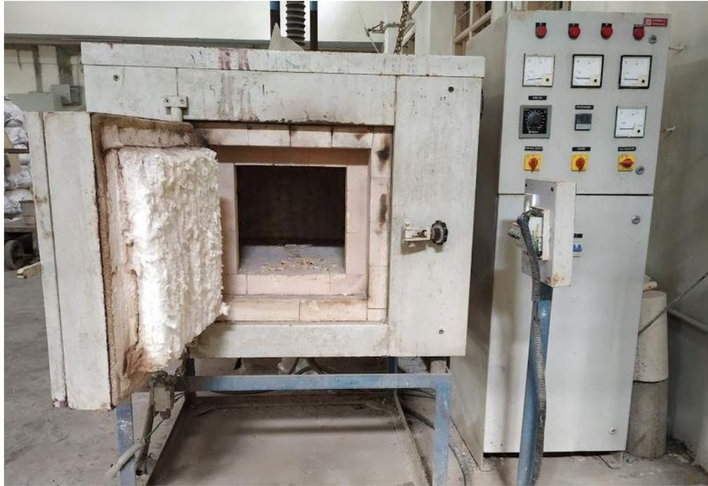
**Fig 6.1 Temperature controlled electric furnace used in the present study**
