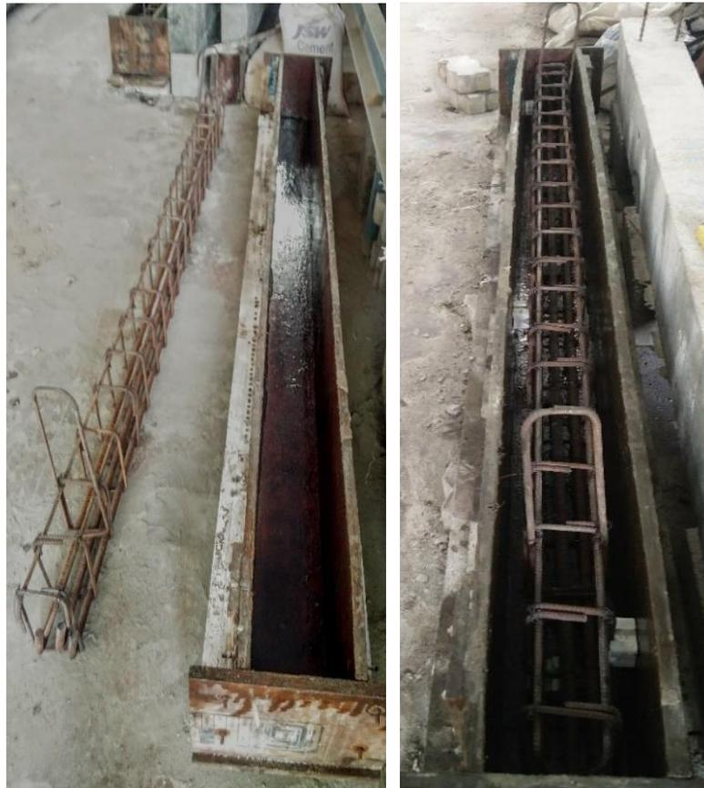
**Fig 8.2 Formwork and reinforcement cage used for casting the beam specimens**
