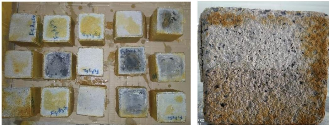
**Fig 5.2 HSAASC mixes after being exposed to sulphuric acid attack for 365 days**
