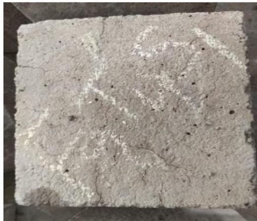
**Fig 6.5 Typical HPAASC specimen after being exposed to 800°C – A closer look**
