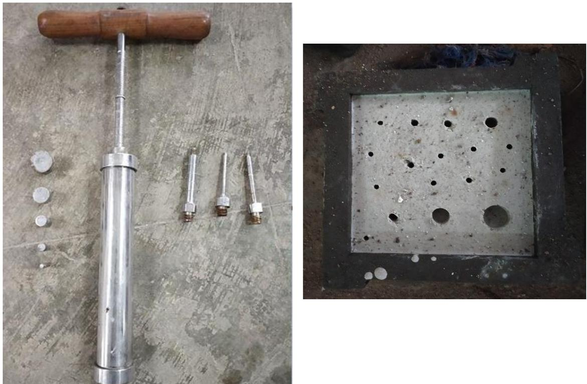
**Fig 4.6 Penetration resistance apparatus with tested concrete sample**
