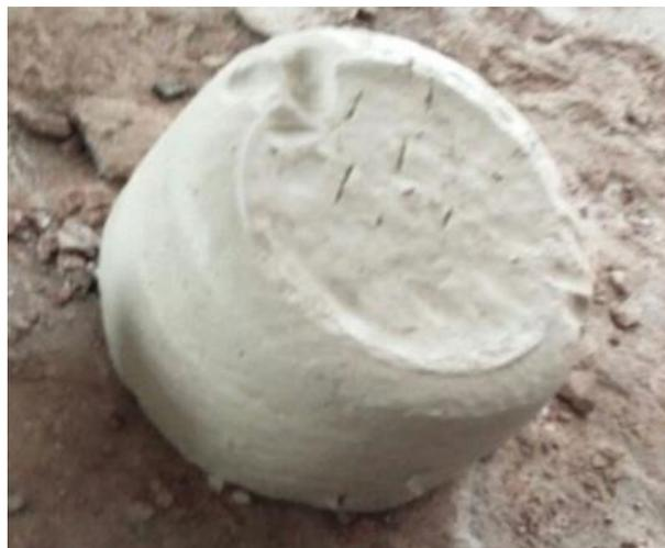
**Fig 4.2 Fast setting behaviour of AASC mix with Lime addition**
