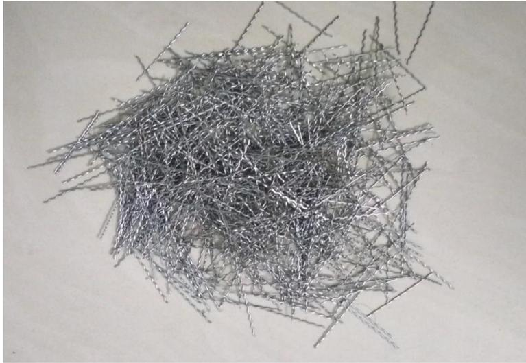
**Fig 7.1 Corrugated Steel Fibers used**
