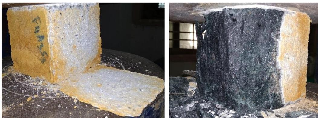
**Fig 5.3 HSAASC mixes exposed to 5% H<sub>2</sub>SO<sub>4</sub> solution, before and after the tests – (Age - 365 days)**
