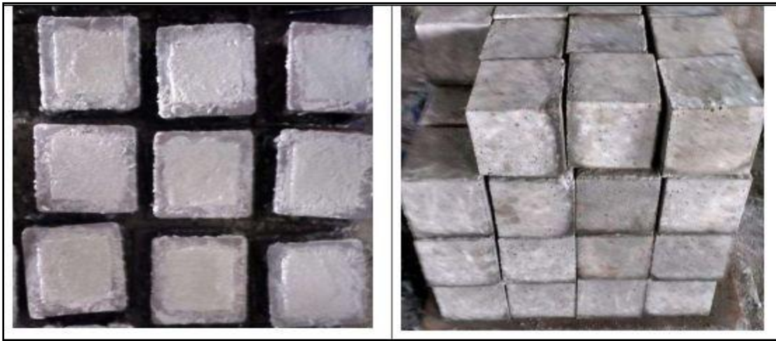
Fig. 3.7 Concrete cubes after casting and demoulding
