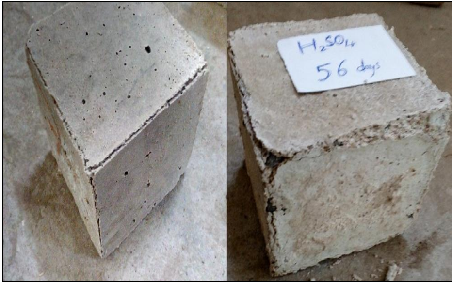
Fig. 6.17 Surface cracks and pop outs on AASC specimens immersed in sulphuric acid
