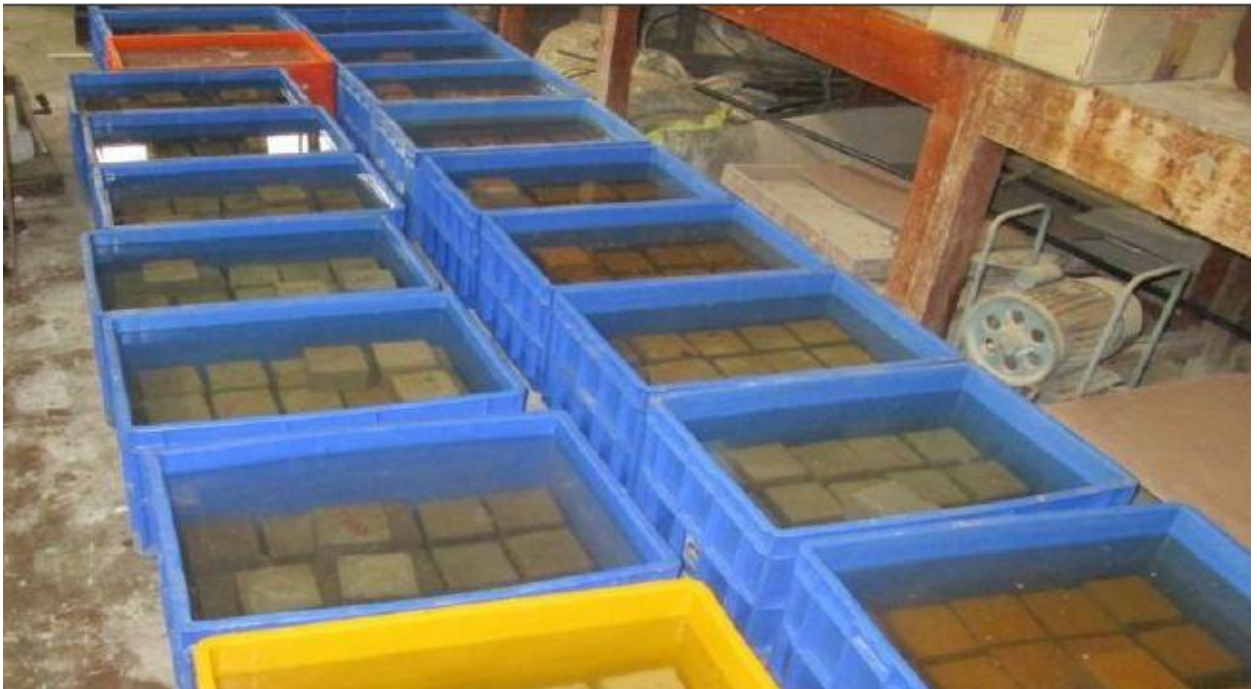
Figure. 6.4 Cubes immersed in acid solution for durability test
