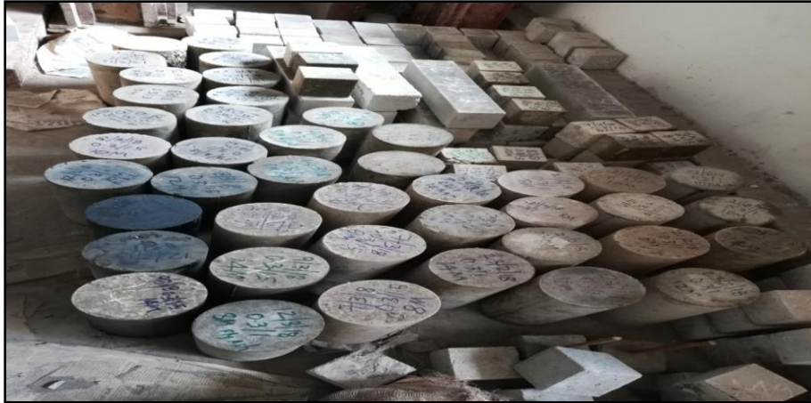
Fig. 3.6 Alkali activated samples kept for air curing.
