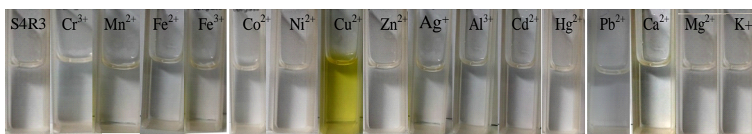
Fig. 4.17: Colorimetric selectivity of S3R3 ( 2.5 \times 10^{-5} M) after the addition of 3.0 equivalences of a different metal cation and 2.0 equivalences of \text{Cu}^{2+} ions
