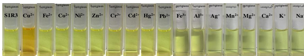
Fig. 2.11: The colorimetric changes observed by naked-eye of chemosensor S1R1–S1R3 upon the addition of 2.0 equiv. of various cations in an aqueous solution
