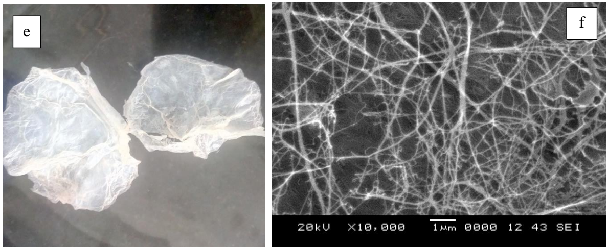
Figure 4.17 BC films with morphological features (a) and (b) air-dried BC films, (c) and (d) BC films oven dried and (e) and (f) freeze dried BC films respectively.
