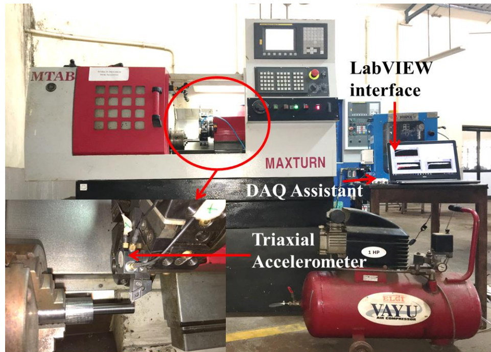
Figure 3.8 The vibration measurement set up for fetching cutting vibration signals
