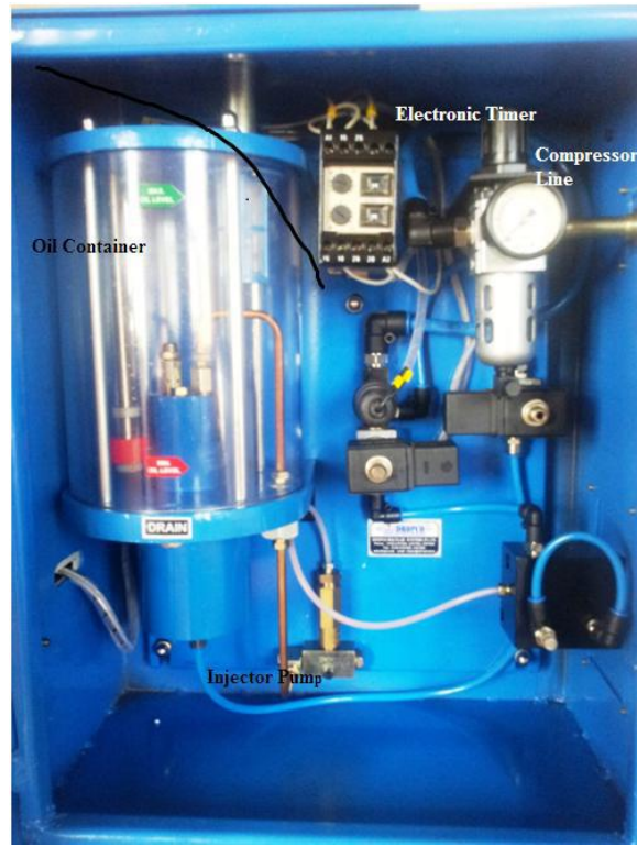
Figure 3.2 Minimum Quantity Lubrication Systems
