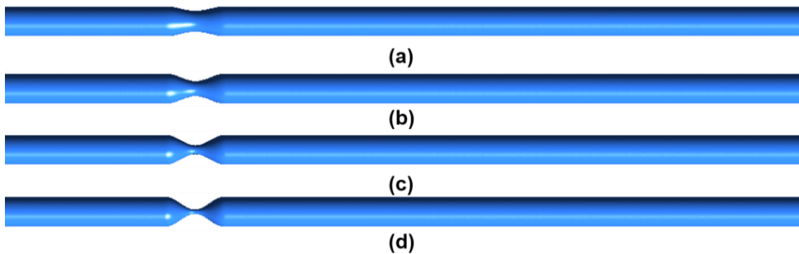
Figure 3.2 Idealized stenosis vessel geometries for different DOS severity, a). 30%, b). 50%, c). 70%, and d). 85% stenosis
