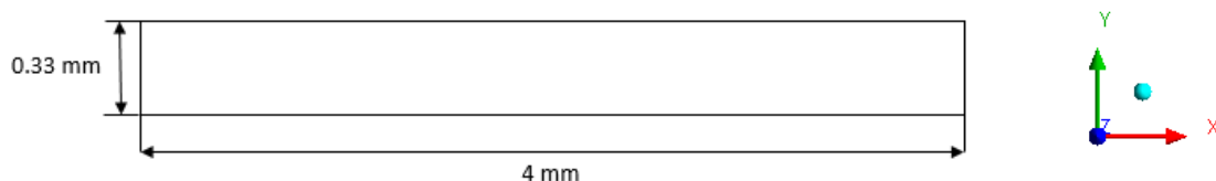
Figure 4.4 Rectangular micro-channel flow system, with depth 100 \mu\text{m} in z-direction (Patrick et al. 2011)
