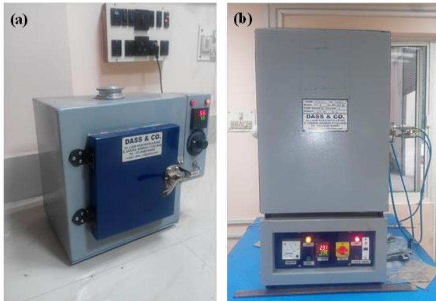
Figure 2.6 Debinding furnace a) Drying oven b) Thermal debinding furnace
