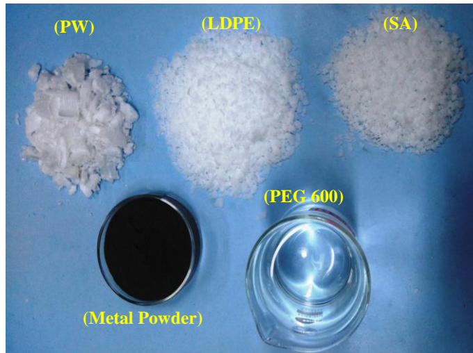
Figure 2.1 Binders for preparation of the feedstock
