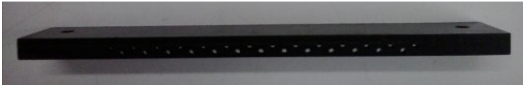
Fig. 3.15 Photograph of fabricated machined Ring 2 with two rows of holes
