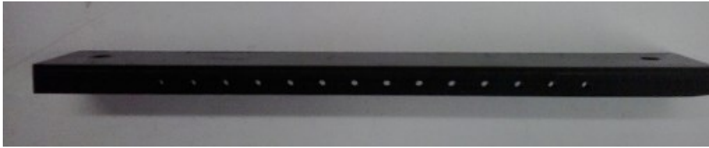
Fig. 3.14 Photograph of fabricated machined Ring 1 with one row of holes
