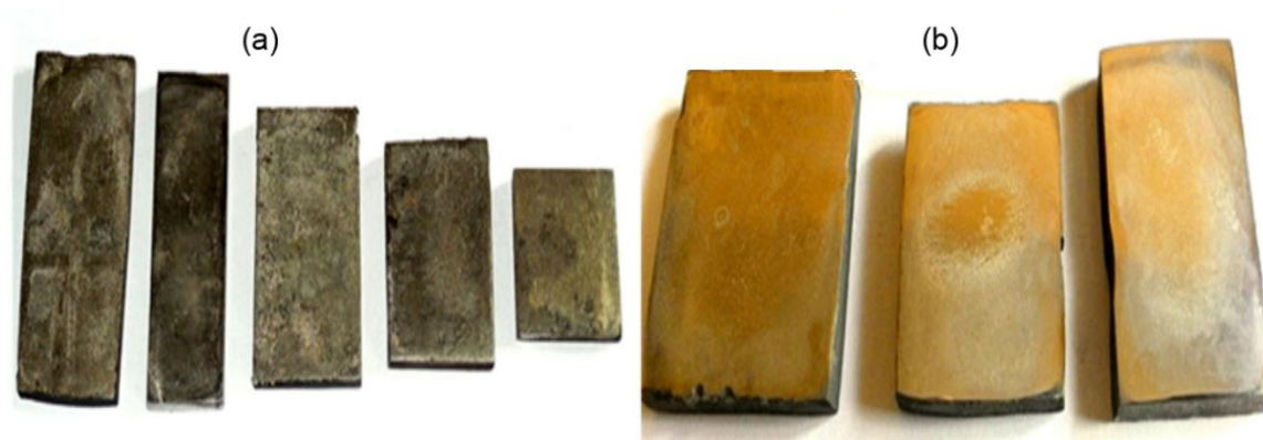
Figure 2.11 (a) Microwave induced EWAC clad samples (b) Clad samples prepared for metallurgical observations (Hebbale and Srinath, 2016)
