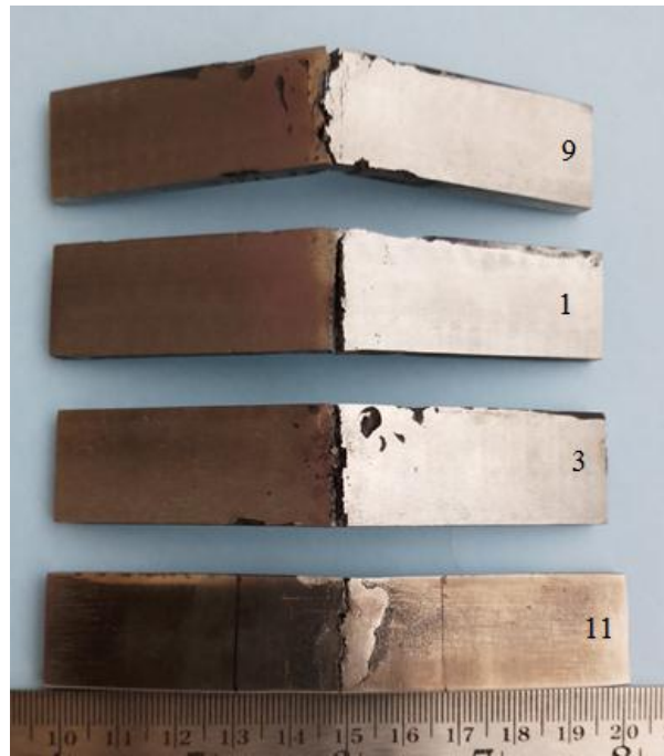
Figure 4.26 Fractured 3-point bend test specimens processed at 600W
