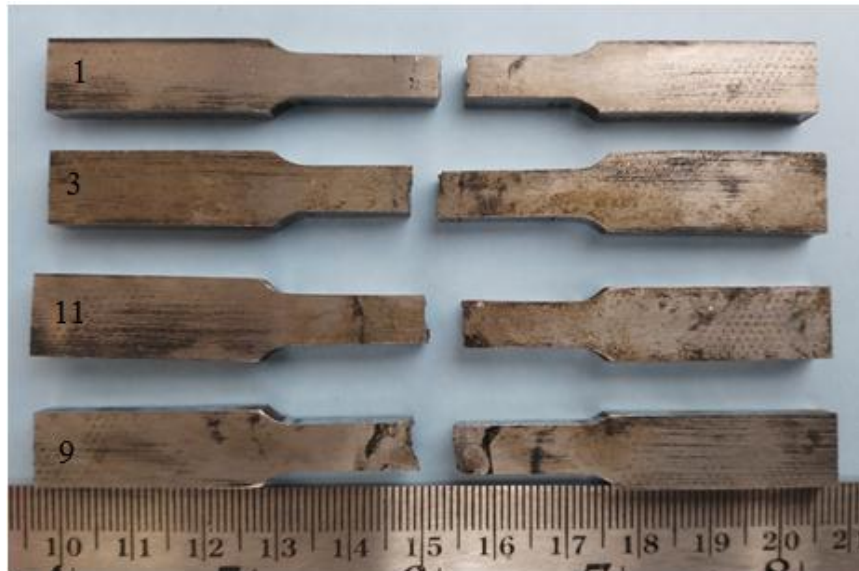
Figure 4.22 Fractured tensile specimens processed at 600W
