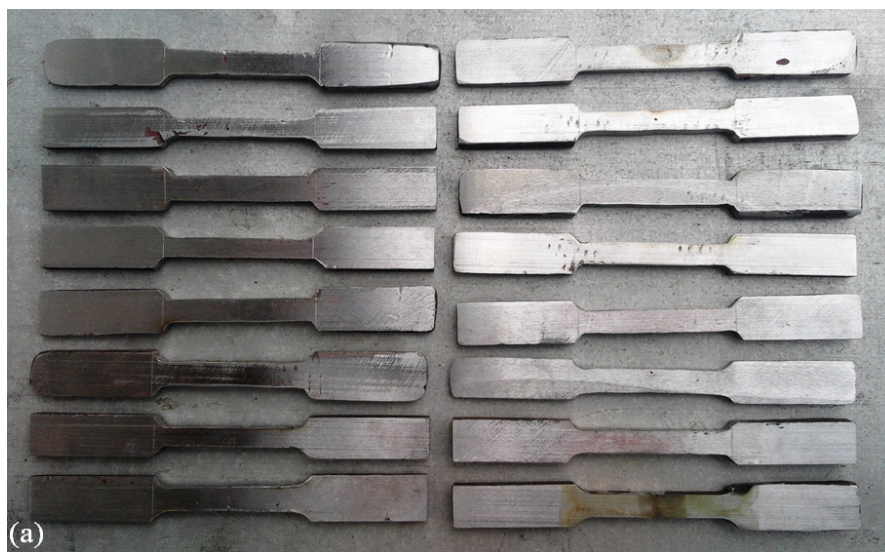
Figure 3.10 ASTM-E8 standard for tensile test specimen
