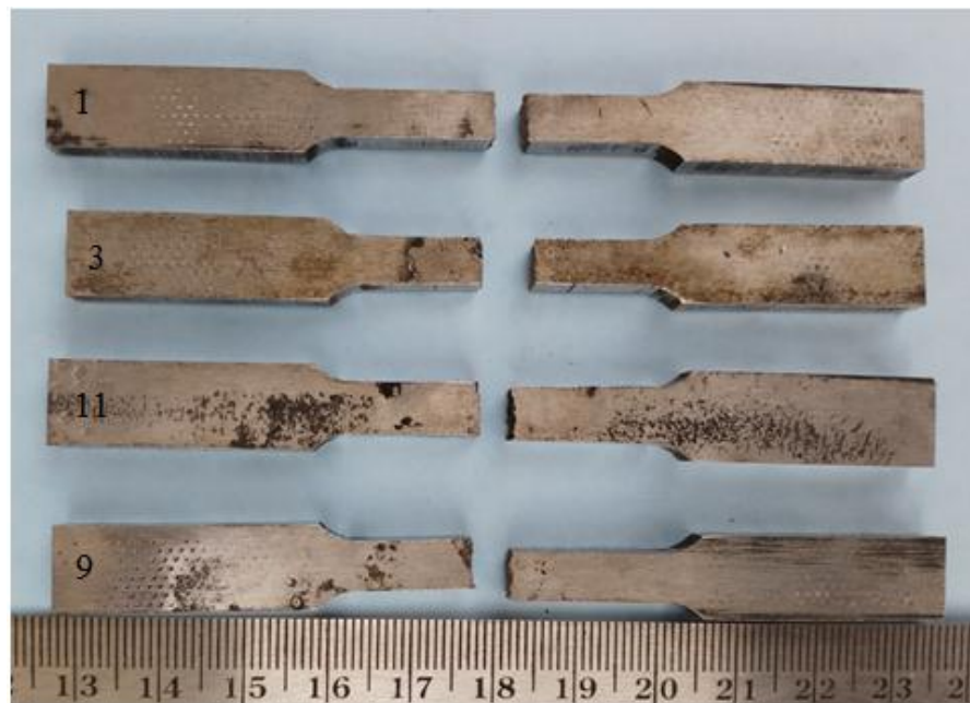
Figure 4.23 Fractured tensile specimens processed at 900W
