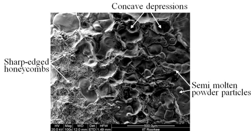
Figure 2.18 SEM micrograph of fractured copper joint (Srinath et al., 2011)
