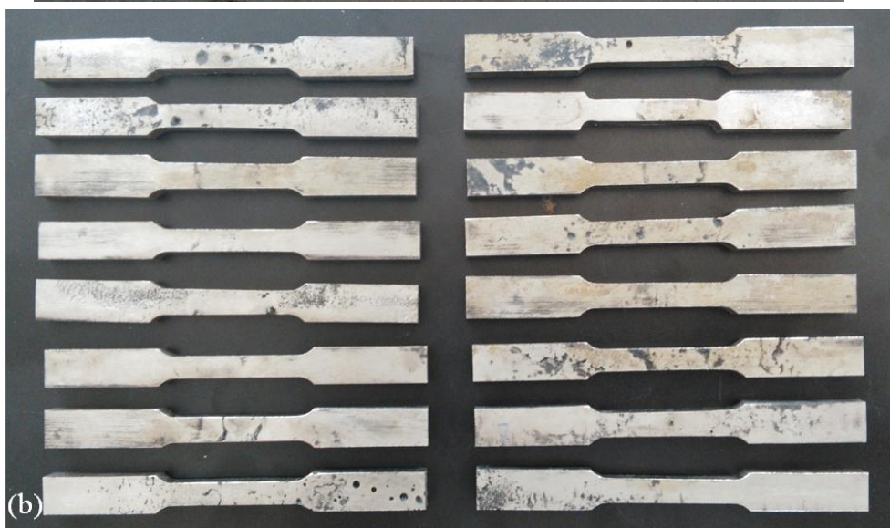
Figure 3.11 Tensile test specimens machined according to ASTM-E8 standards processed at (a) 900W (b) 600W
