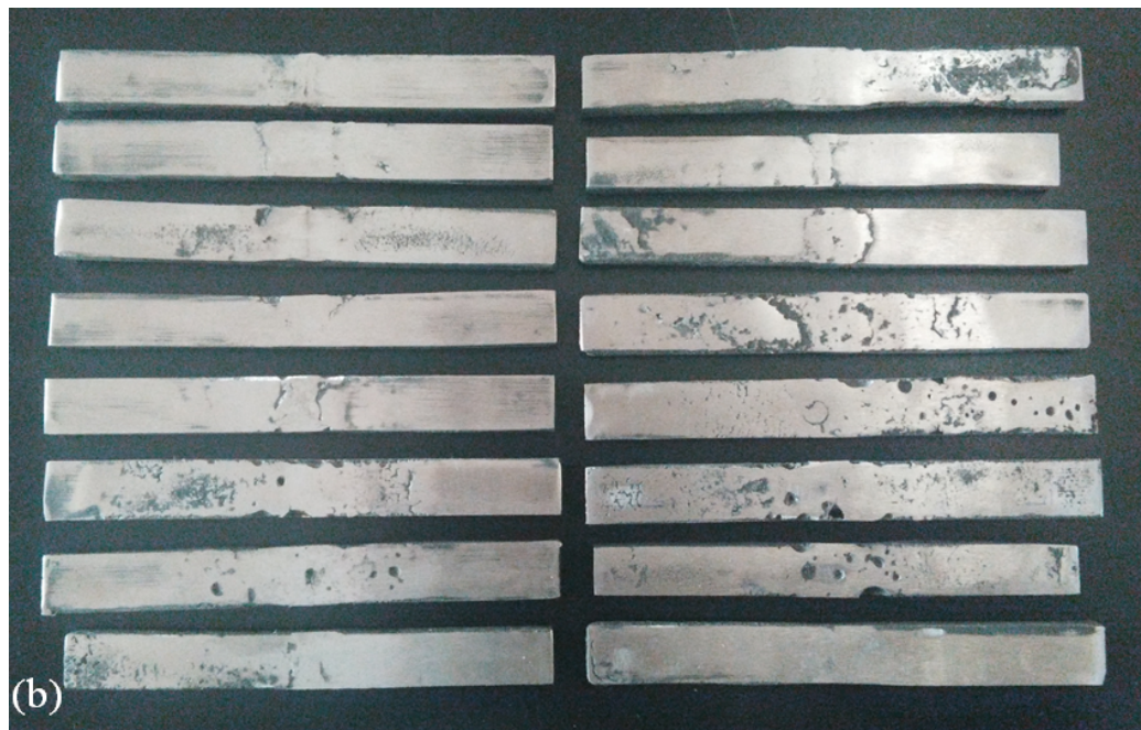
Figure 3.9 Specimens processed at (a) 900W (b) 600W power after polishing
