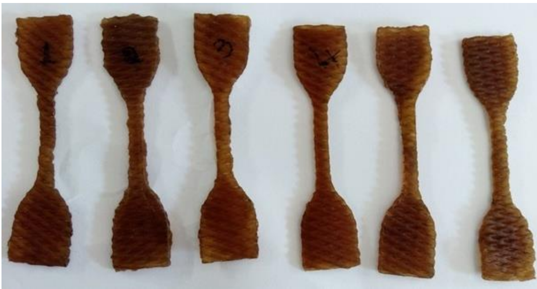
Figure 2.21 Natural rubber tensile test samples
