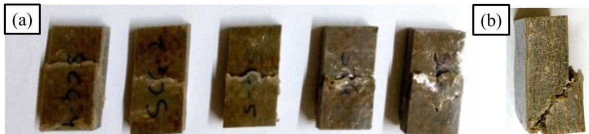
Figure 3.25 JEF composites fractured failed samples by shear in compression (a) top view, and (b) side view
