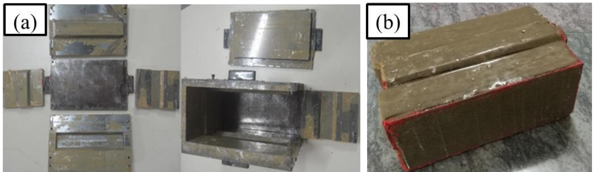
Figure 2. 29 (a) Mold used for producing interlock block, and (b) A sample of interlock block
