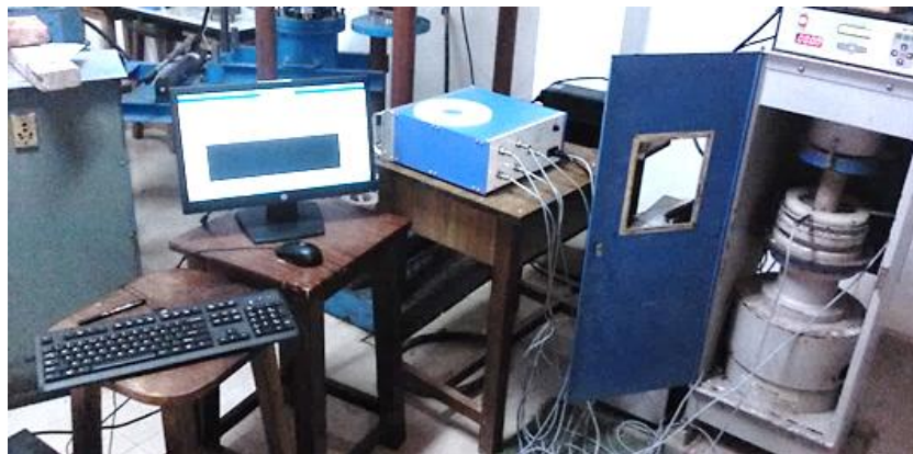
Fig. 3.37 PC based DAQ system integrated with compression testing machine
