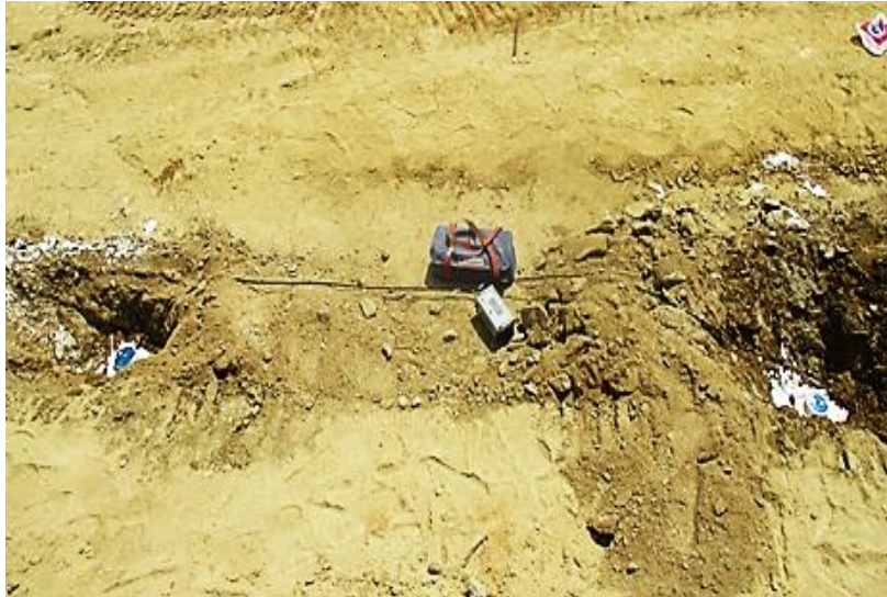
Fig. 3.21 Monitoring of ground vibrations in granite stone formations at different locations during research field studies
