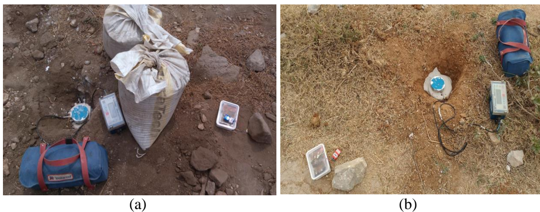
Fig. 4.35 Vibration capturing with vibration monitor and developed piezo generator circuit in granite formation
