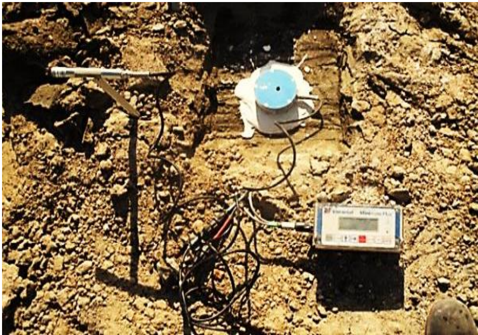
Fig. 3.19 Monitoring of ground vibrations in sandstone bench formations at different locations during research field studies
