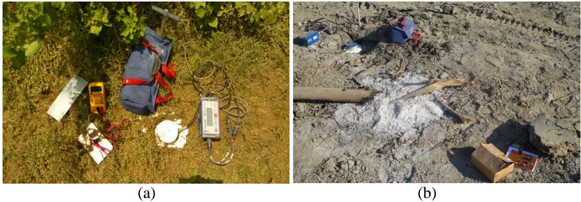
Fig. 4.32 Vibration capturing with vibration monitor and developed piezo generator circuit in sandstone formation
