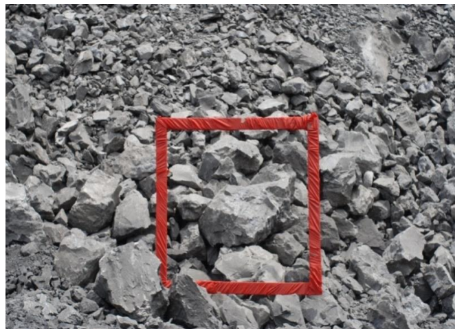
Fig. 2.2 Fragmented muck pile captured with 0.5m x 0.5m calibrator
