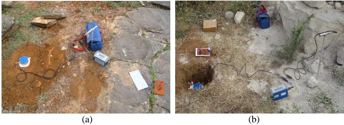
Fig. 4.22 Vibration capturing with vibration monitor and developed piezo generator circuit in limestone formation
