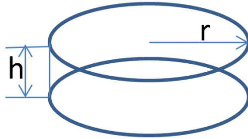
Figure 1 Schematic representation of perfect nucleus of disc shape having radius 'r' and height 'h'.
