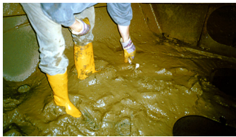
(a) Drilled mud \tau_0 = 15\text{Pa}
