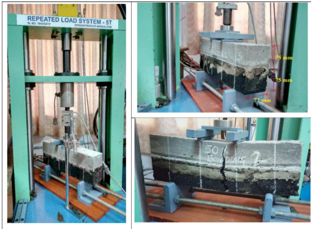
Fig. 4.2 Represents the repeated load test for HMA-UTW composite prism specimens and 50 % interface bonding failure specimen
