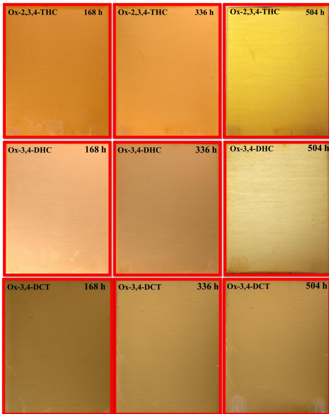
Figure 3.38 Photographs of Ox-2,3,4-THC, Ox-3,4-DHC, and Ox-3,4-DCT coupons after salt spray exposures.
