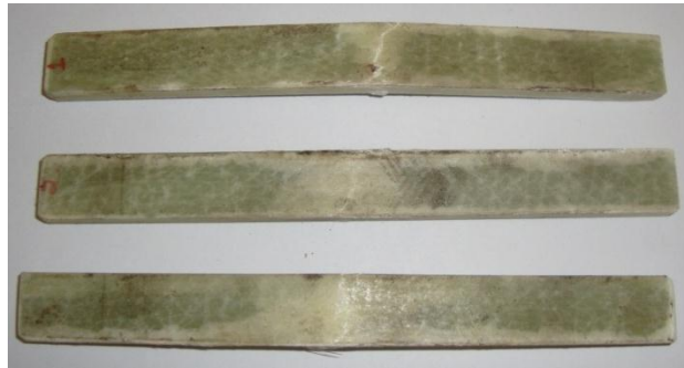
Fig.4.5(b).Photograph showing typical failure observed in flexural test of GE pultruded samples
