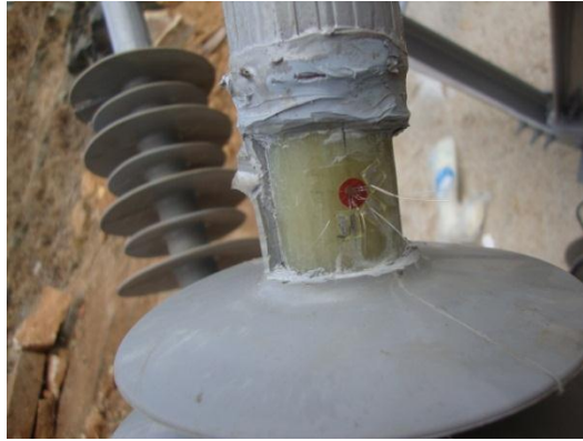
(a) Photograph of a typical strain gauge mounted on GE pultruded rod of cross arm
