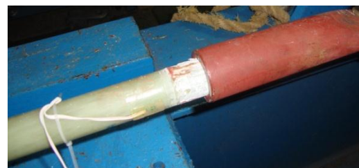
(e) End clamps with adhesive bonding slipping early during loading
