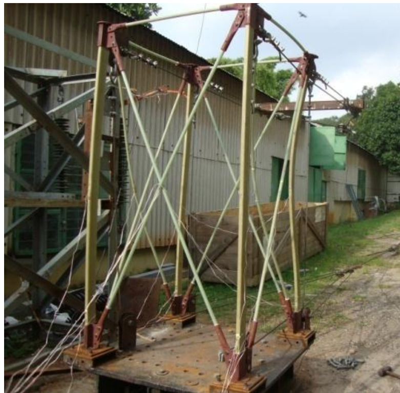
Fig.4.14 Photograph showing buckling of leg and bracing of tower sub assembly prototype TS1 during testing
