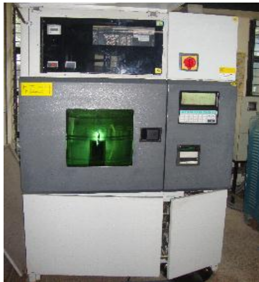
Fig 3.6a Test set up of accelerated weathering test
