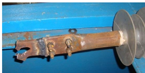
(d) End clamps with crimping remaining intact after loading
