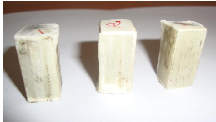
Fig.4.3 Typical failure modes in compression test
