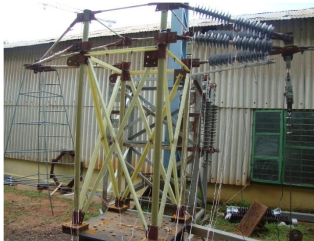
Fig. 3.23 Photograph showing mechanical testing of X-braced tower unit with cross arm prototype TSCA2.
