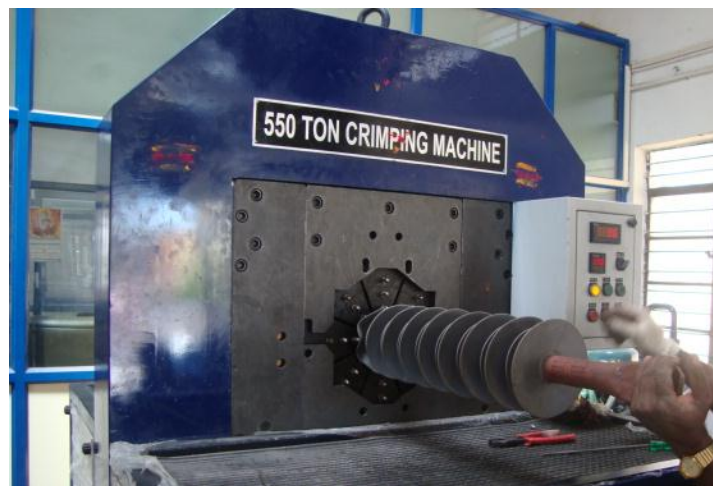
Fig 3.15 Crimping machine set up
