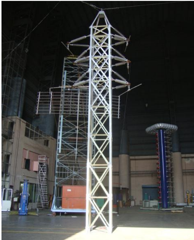
Fig 3.38 ( c ) Photograph showing live conductor attached to the cross arm with composite member with 15 m tower
