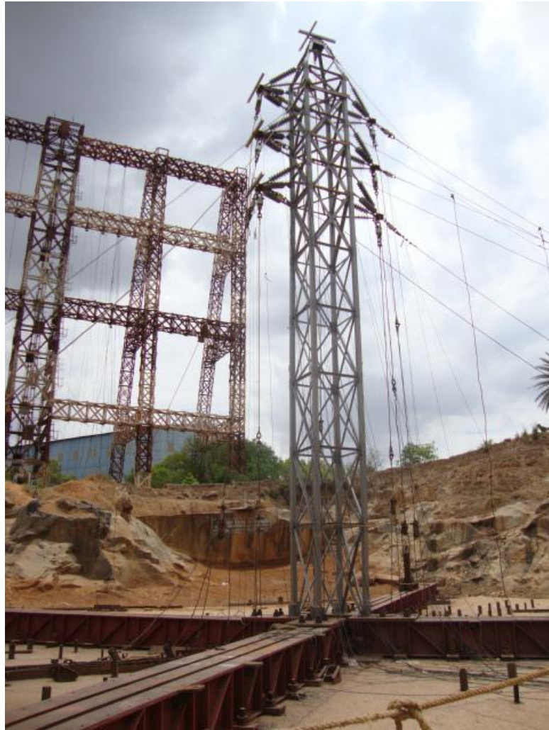
Fig 3.33 Photograph showing the tower and the loading arrangements
