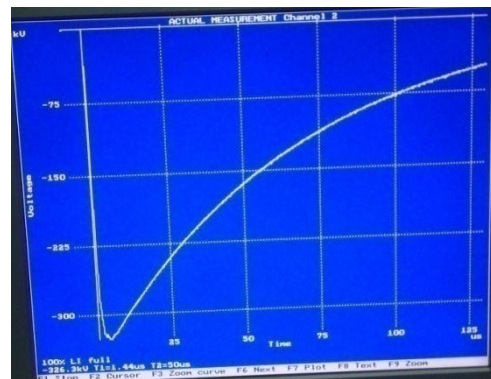
(e) Snap shot of lightning impulse voltage/time curve (-ve polarity) for cross arm
