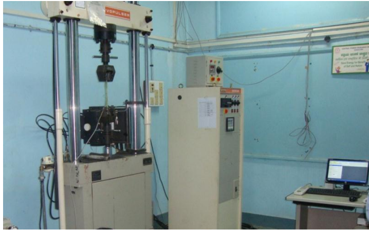
Fig.3.3 Photograph showing tensile strength test set up
