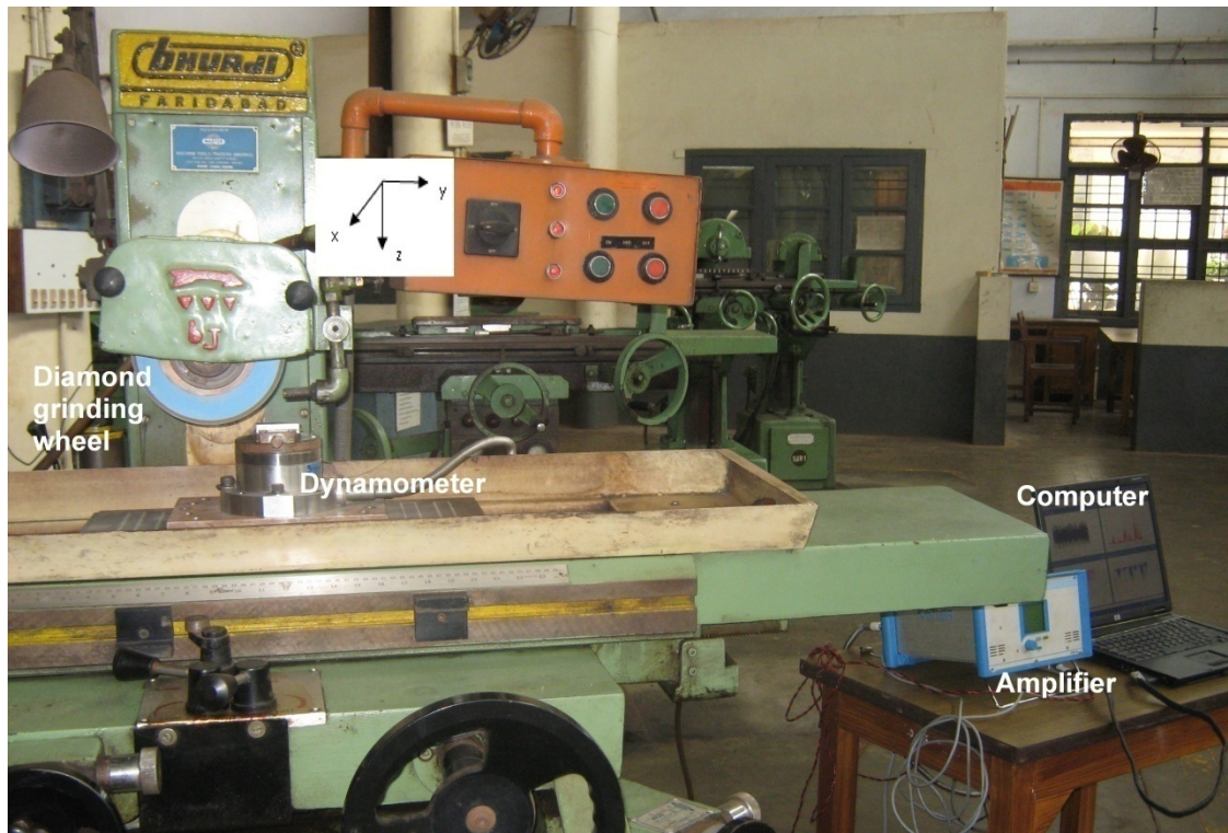
Figure 3.5 Kistler dynamometer setup
