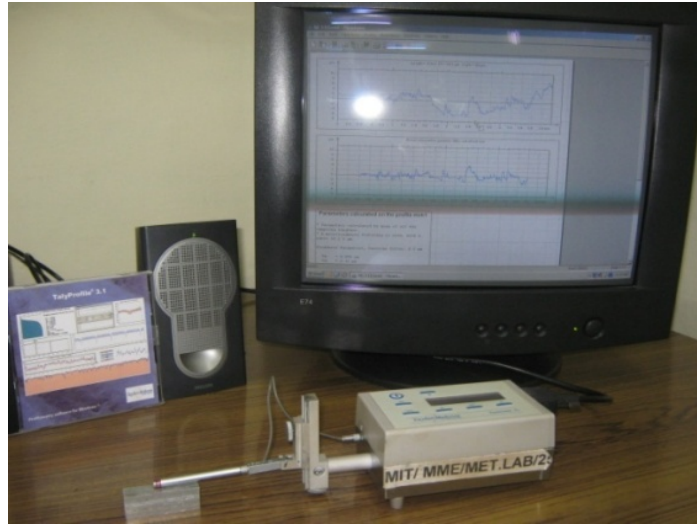
Figure 3.7 Roughness measuring Instrument
