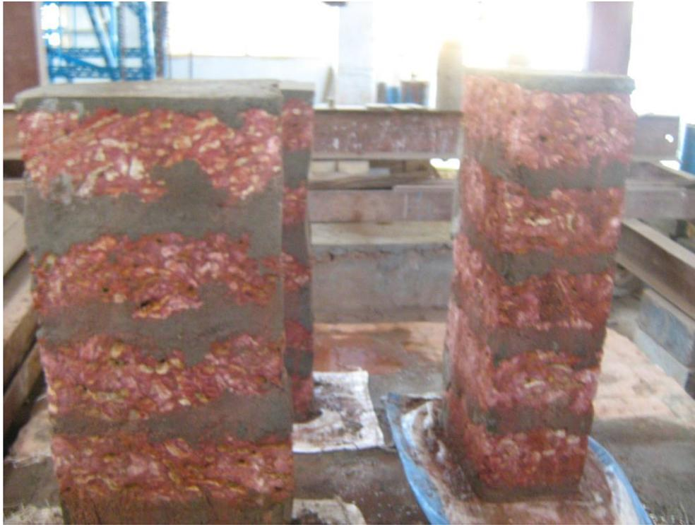
**Fig. 3.7 Laterite masonry prisms cast for testing**
