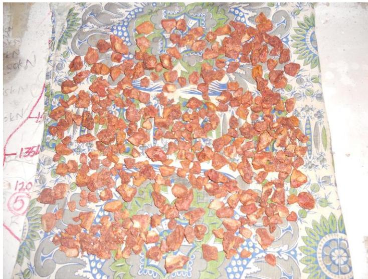
**Fig. 3.5 Laterite sample for water absorption & specific gravity**
