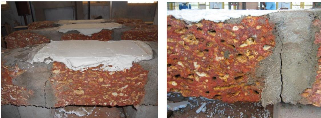
**Fig. 3.12 Shear bond failure of laterite masonry triplets (scheme A)**
