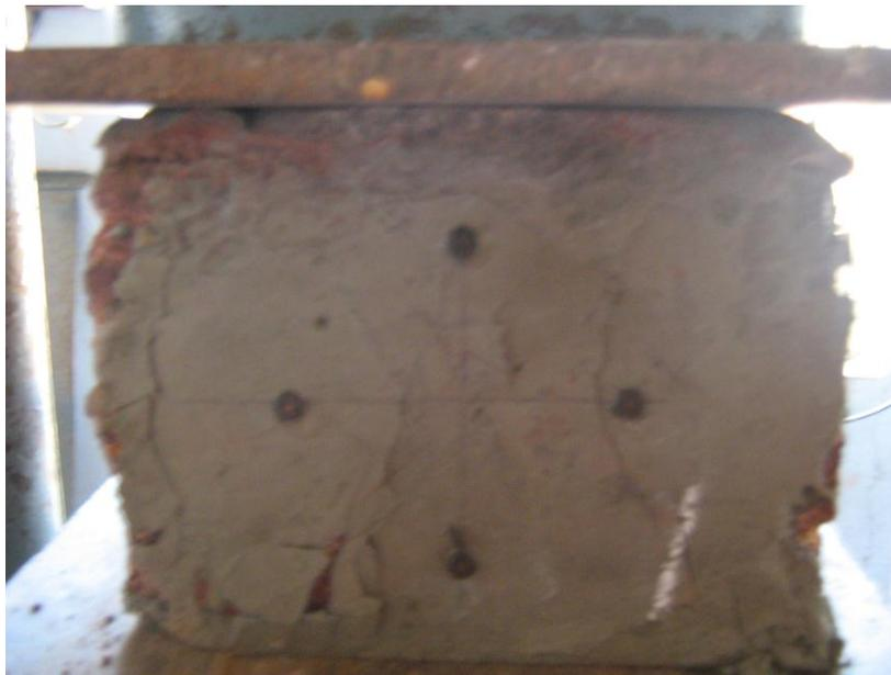
**Fig. 3.3 Demec buttons glued on laterite blocks**
