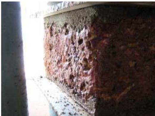
**Fig. 3.1 Laterite block capped with cement mortar for compression test**
