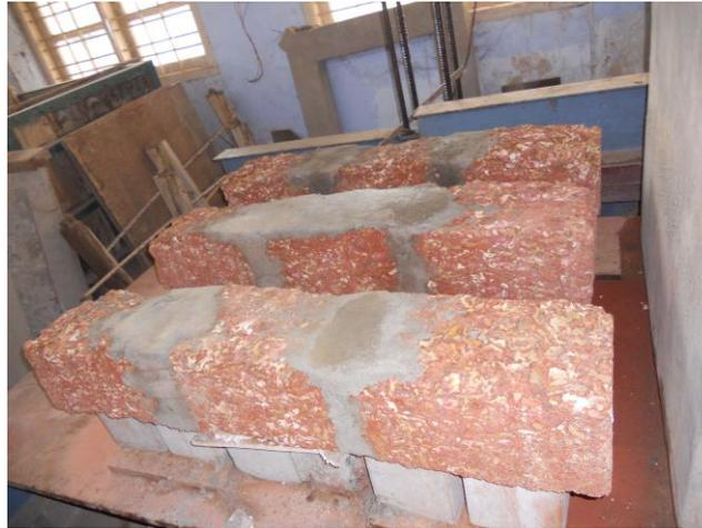
**Fig. 3.11 Laterite masonry triplets cast for testing (scheme A)**
