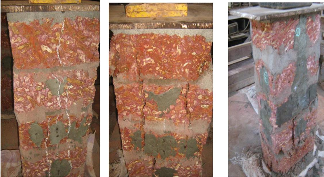
**Fig. 3.8 Failure of stack-bonded laterite masonry prisms**
