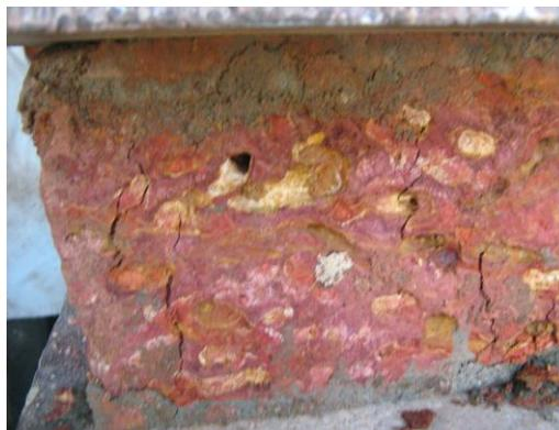
**Fig. 3.2 Failure pattern in laterite under compression**
