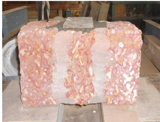
**Fig. 3.13 Laterite masonry triplets (scheme B)**
