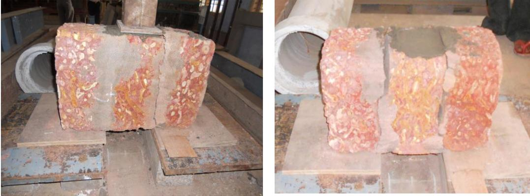
**Fig. 3.14 Shear bond failure of laterite masonry triplets (scheme B)**
